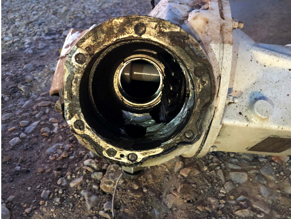
Figure 18: 90-degree Gearbox Attachment Points
