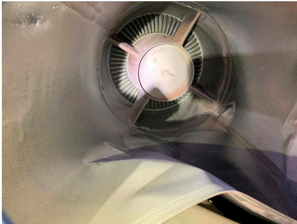
Figure 11: Metal Spray on Turbine Blades
