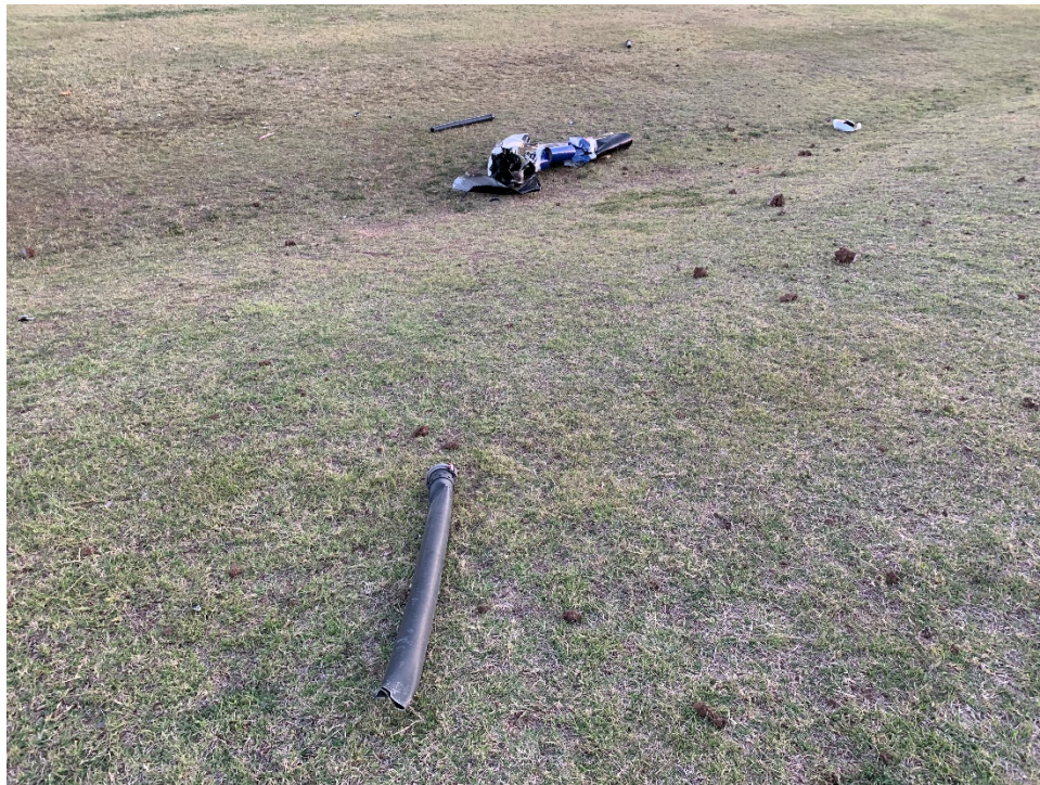
Figure 13: Aft Tail Rotor Driveshaft in Relation to Vertical Stabilizer
