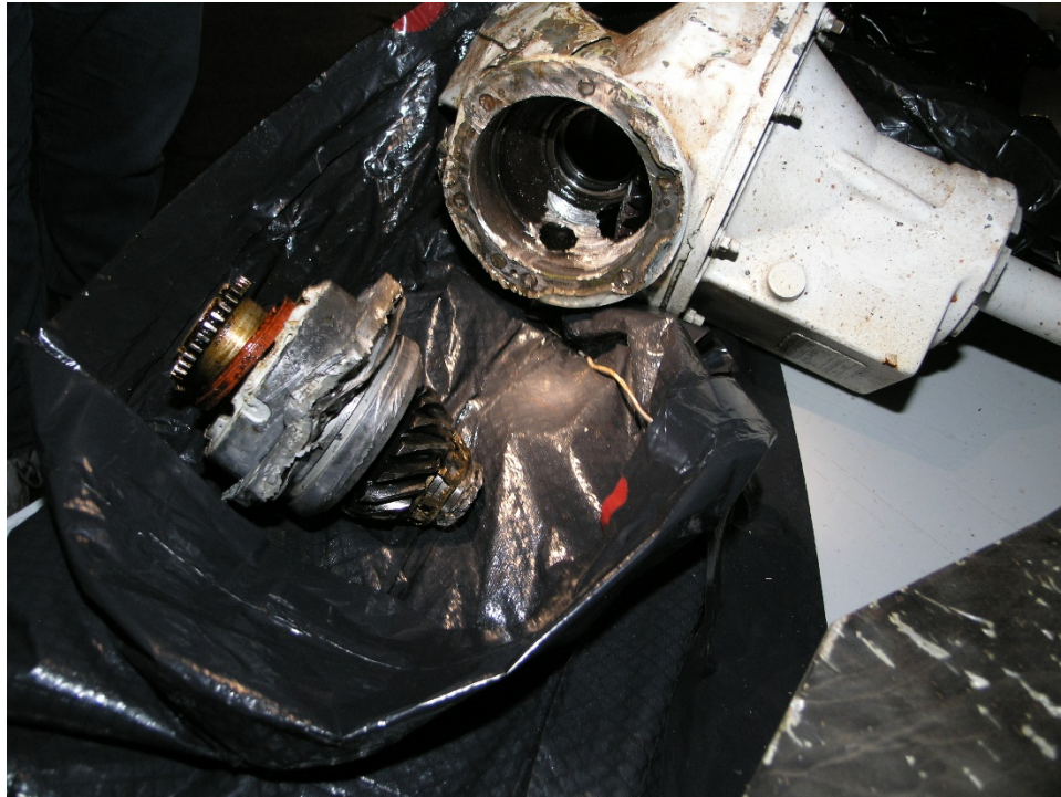
Figure 20: The Input Quill Gear next to the 90-degree gearbox
