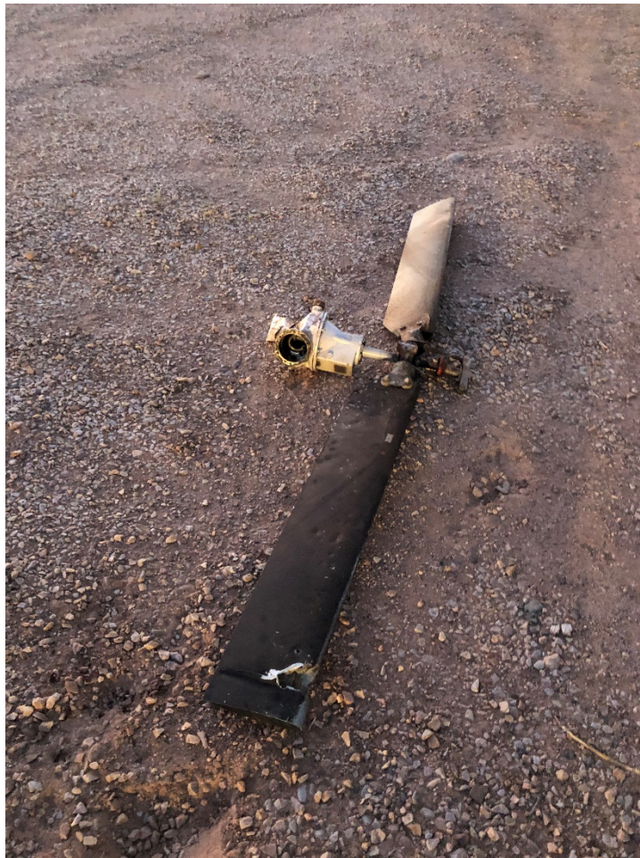
Figure 17: The 90-Degree gearbox and Tail Rotor Assembly
