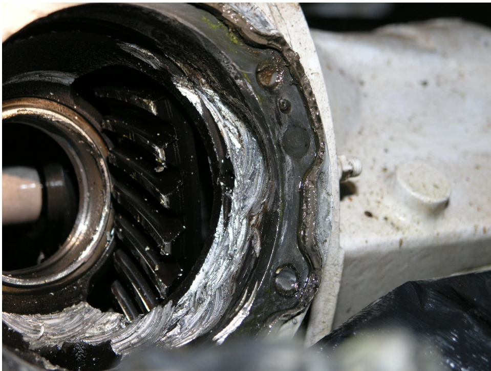
Figure 19: Rotational Scoring on the 90-degree Gearbox Housing
