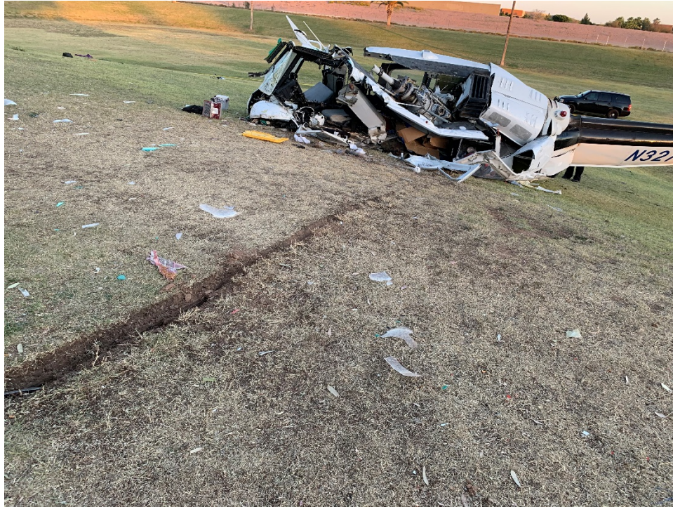
Figure 6: Main Rotor Blade Strike
