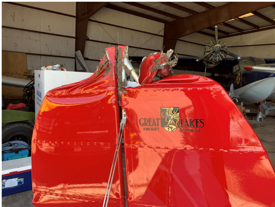
Figure 4: Vertical and Rudder Damage
