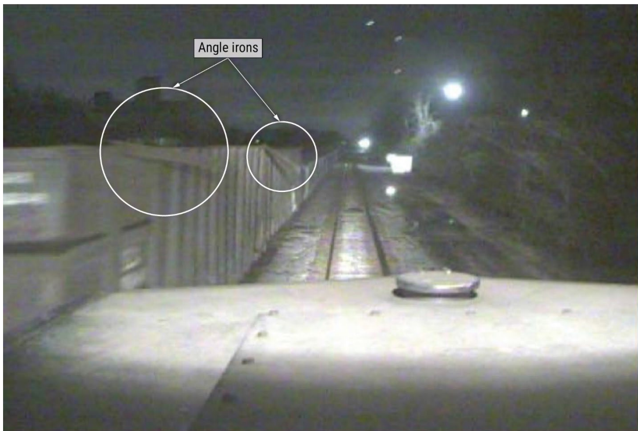
Figure 2. Gondola car and protruding angle iron section immediately before impact. (Source: NS.)
