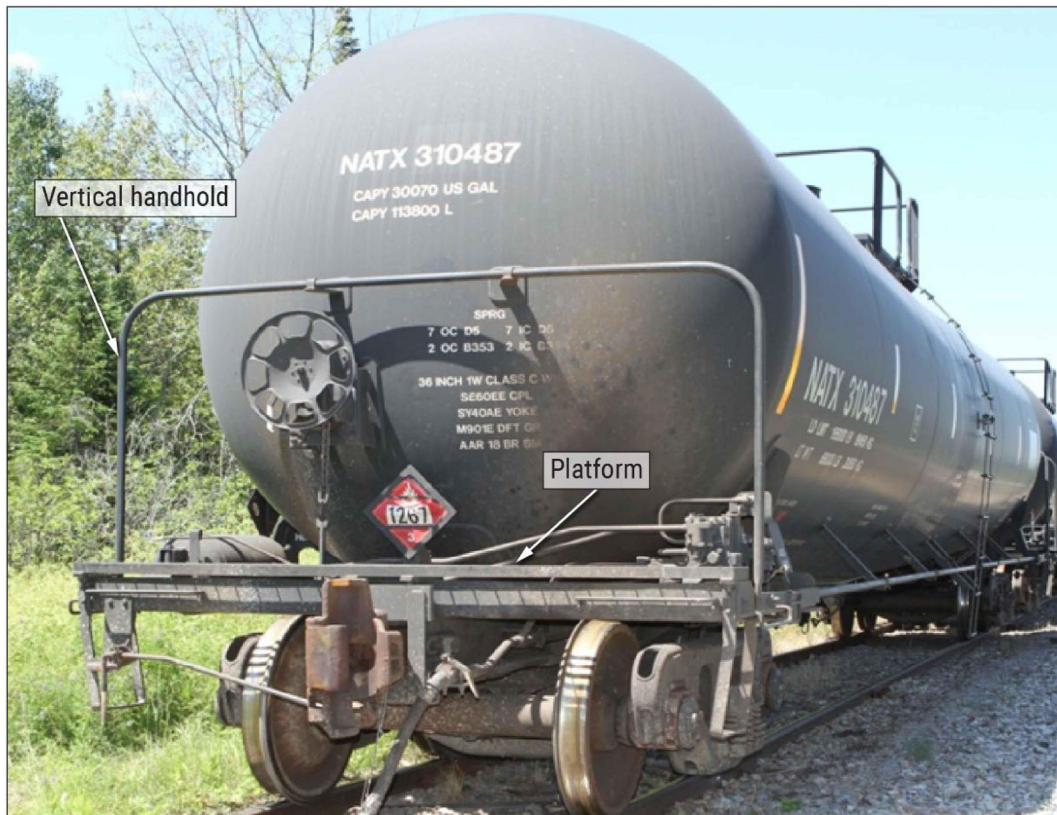
Figure 2. Exemplar tank car depicting the vertical handhold and platform. (Source: Transportation Safety Board of Canada.)
