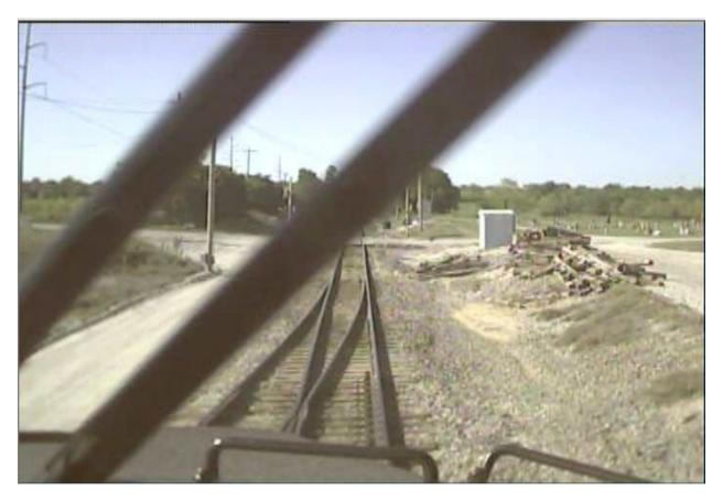
Image from the NS 4055, lead unit on the RHKPHQ15, as it traversed the C yard switch on arrival at Chico. This confirms that the crew that moved the RDACO14 in the C yard lined the C yard switch back for main track movement when they were complete.
