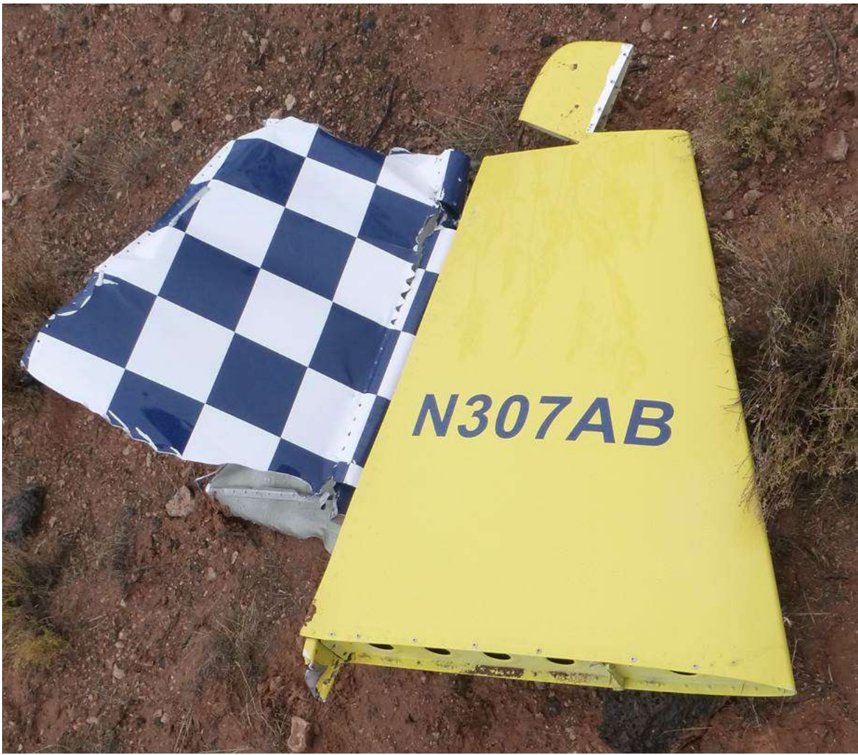
Figure. Vertical stabilizer and attached rudder.
