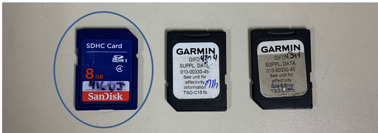
Figure 2. SD card containing flight data (left, circled).
