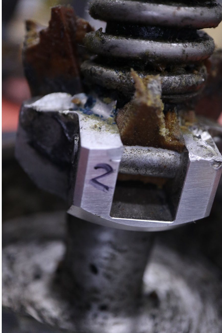
Figure 3. View of the Fractured Phenolic Blade Actuating Link for the No. 2 Propeller Blade.
