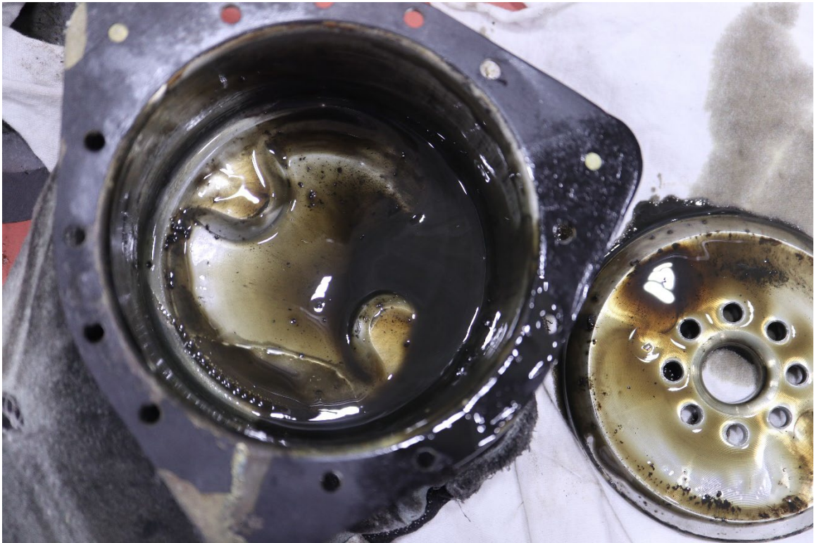
Figure 6: View of the Residual Oil in the Cylinder.
