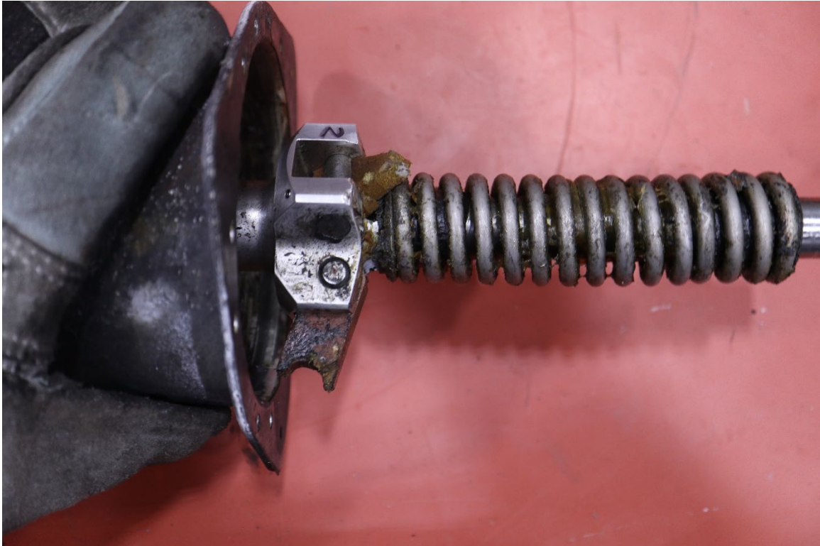
Figure 4: View showing the spring and piston on the low Pitch.
