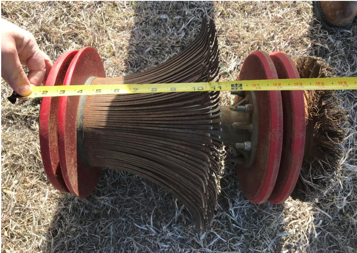
Figure 4. Photograph of the 10-inch PitBoss™ Cleaning Pig that Impacted Technician 1 Rodriguez, March 28, 2020
