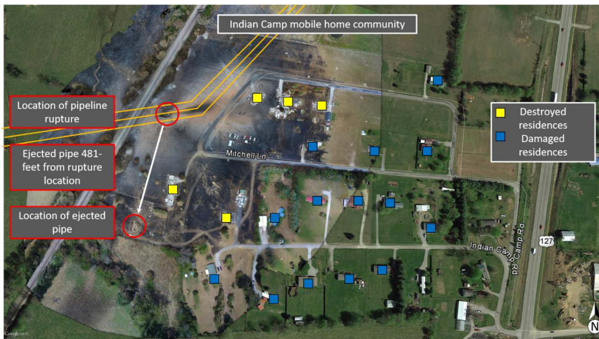
Figure 1. Postrupture aerial view of the accident area. (Photo overlaid on Google Earth image.)
