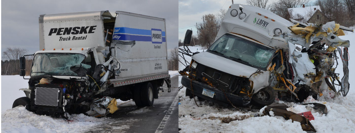
Figure 1. Photo showing both crashed vehicles at final rest. Front end damage to the 2021 Freightliner straight truck is shown on the left and damage to the driver's side of the 2013 medium size bus is shown on the right. (Source: New York State Police)
