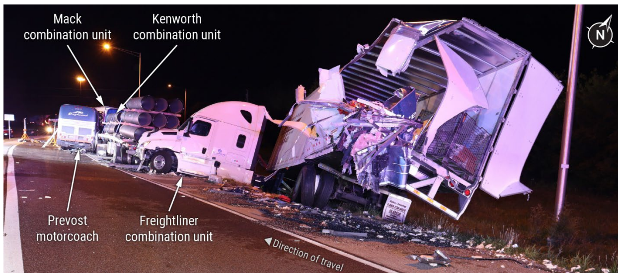
Figure 1. Crash scene photograph showing the motorcoach and three tractor-trailer combination vehicles. (Source: Illinois State Police, annotated by NTSB)
