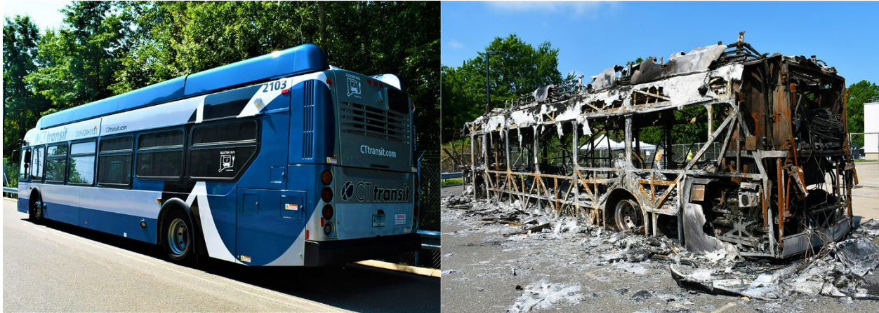
Figure 1. Photo on the left shows an exemplar CTtransit battery electric bus. Photo on the right shows the post-fire damage to the bus involved in the event.
