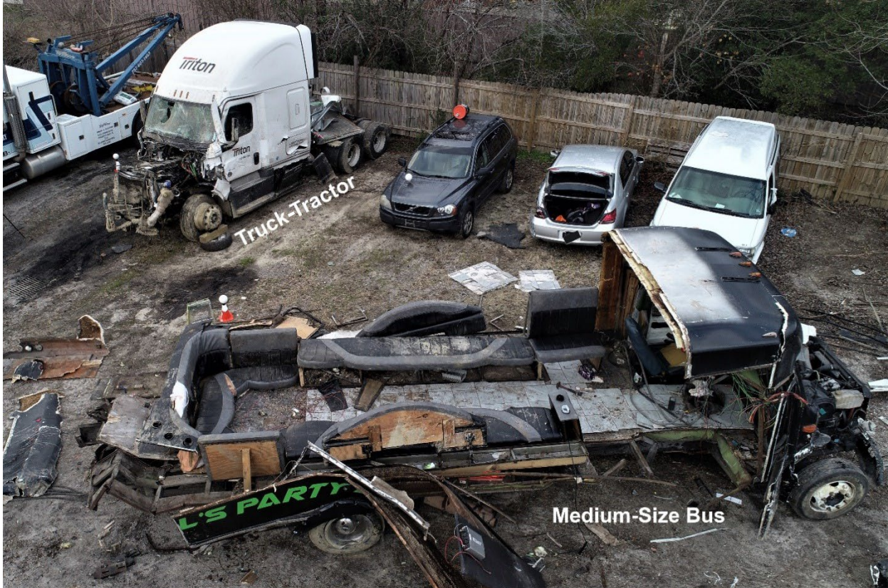
Figure 1. An elevated view showing both vehicles after they had been removed from the crash scene and taken to a tow yard. The medium-size bus is in the foreground. The bus body sustained catastrophic damage in the crash and the interior seating can be seen from this right-side view of the vehicle. The truck-tractor from the combination vehicle is located behind and to the left of the bus, and the significant damage to the front of the vehicle can be seen.
