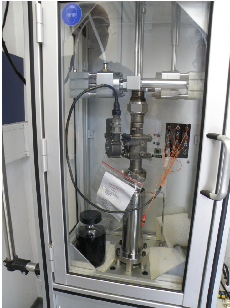
Figure 36: Green FSOV S/N7095 on ATP test stand
