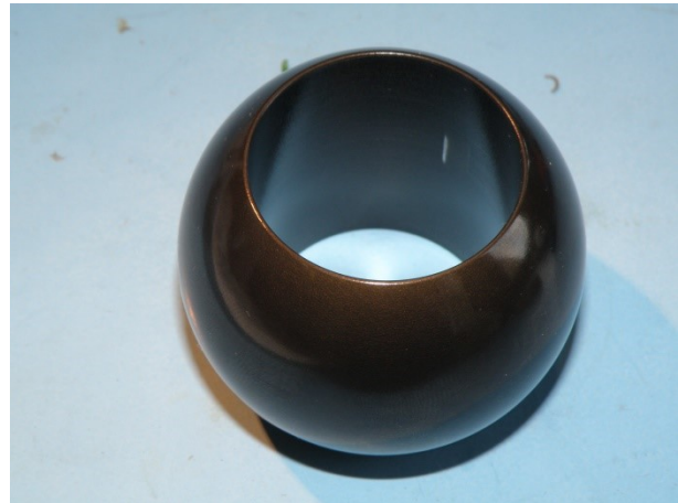
Figure 33: Valve ball with manufacturing marks inside
