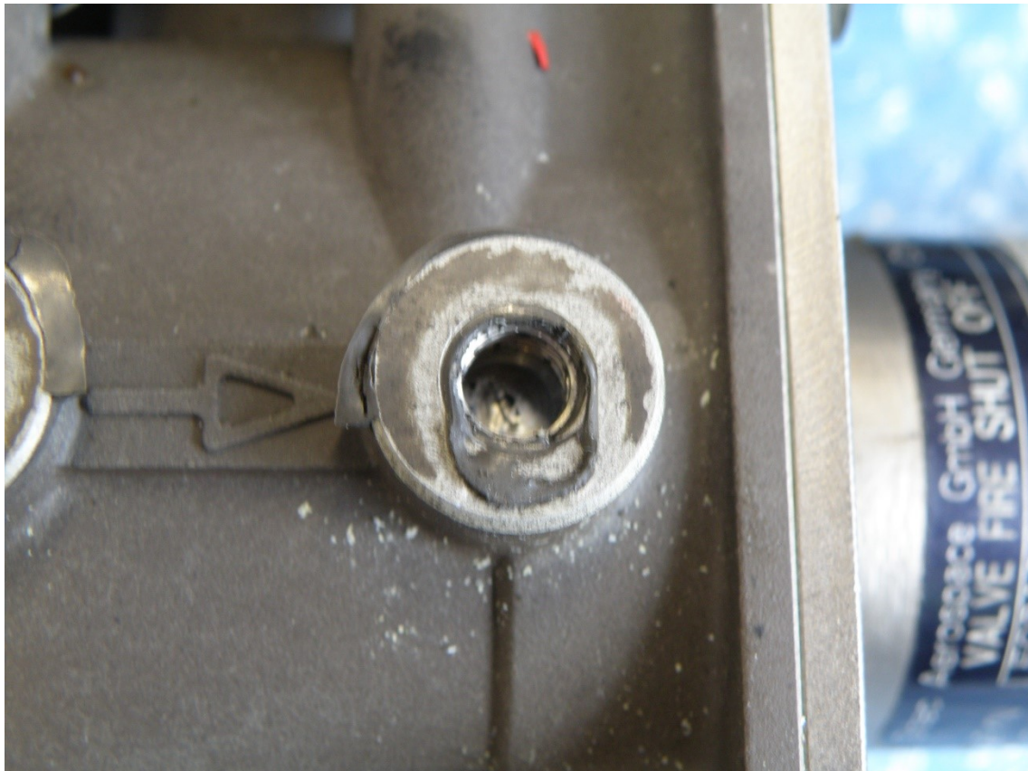
Figure 3: Imprints on mounting hole
