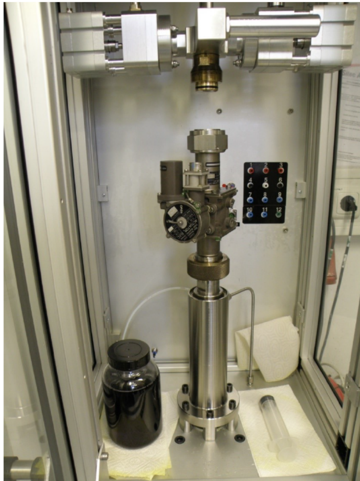
Figure 12: ATP Test Stand with FSOV
