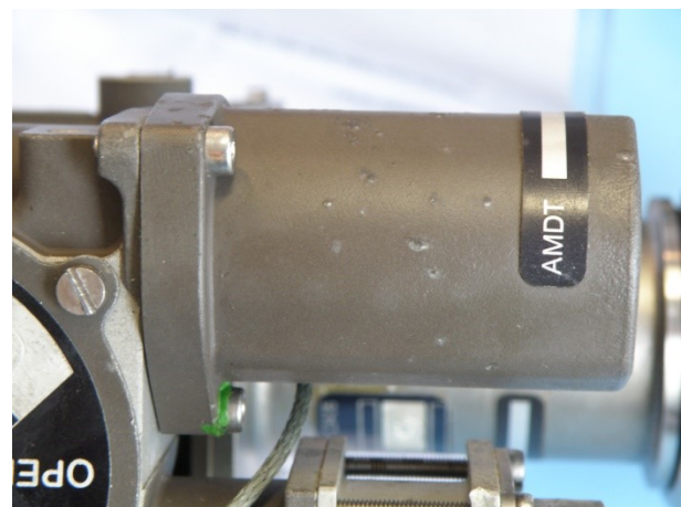
Figure 6: Dents/ Deposits on motor cover 2
