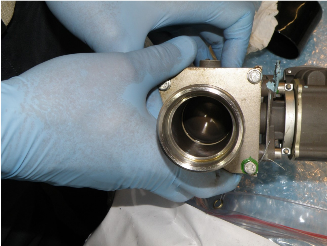
Figure 4: Visual Inspection of Ball Position
