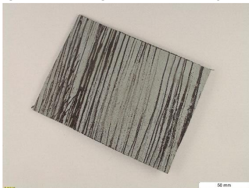
Figure 4. Cowling inner side- Honeycomb sample extracted from the area affected by material loss
