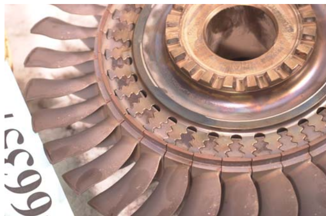
PHOTO 12: ROTATIONAL RUB ON 2 ND DISK
