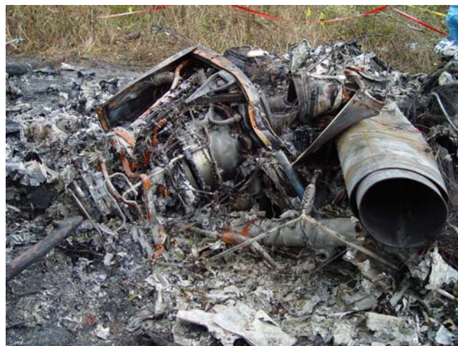
PHOTO 3: RT ENG AT MAIN WRECKAGE SITE
