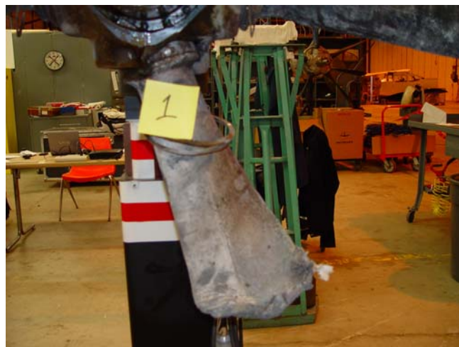
PHOTO 25: BLADE 1 MISSING TIP
