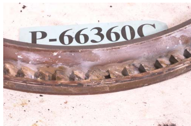
PHOTO 17: DEBRIS IN THE 2 ND -STAGE DIFFUSER
