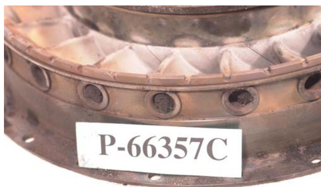
PHOTO 11: DEBRIS IN SHROUD COOLING HOLES
