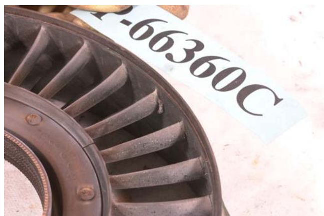
PHOTO 21: METAL SPRAY ON VANE AIRFOILS
