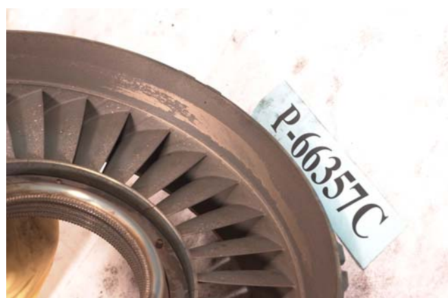
PHOTO 13: RUB & METAL SPRAY ON 3 RD SHROUD
