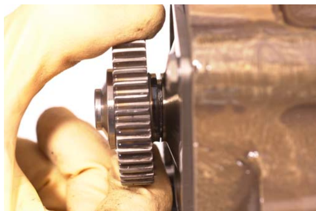
PHOTO 7: FRACTURED TORQUE SHAFT ASSEMBLY
