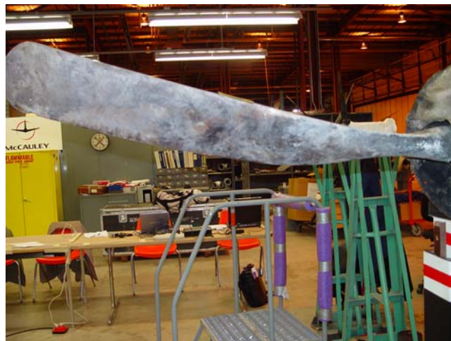
PHOTO 33: BLADE 4 BENT AND TWISTED
