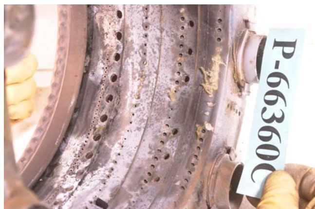
PHOTO 18: DEBRIS LODGED IN COOLING HOLES
