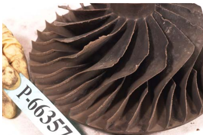
PHOTO 8: 1 ST -STAGE IMPELLER DAMAGE
