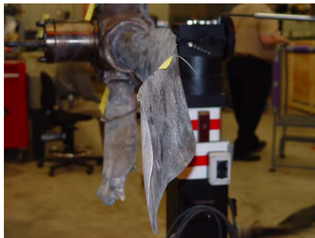
PHOTO 27: BLADE 4 BENT AND CURLED
