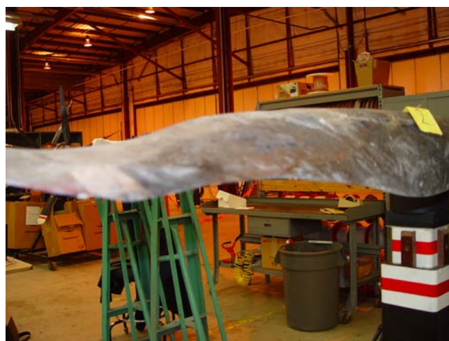
PHOTO 26: BLADE 2 BENT AND CURLED
