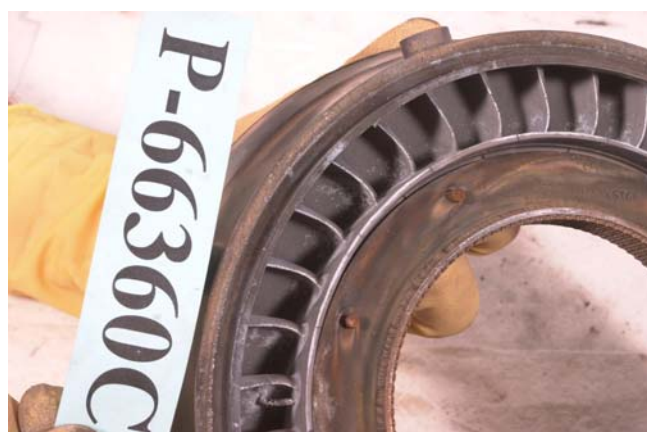
PHOTO 20: FIBROUS DEBRIS IN 2 ND -STAGE NOZZLE
