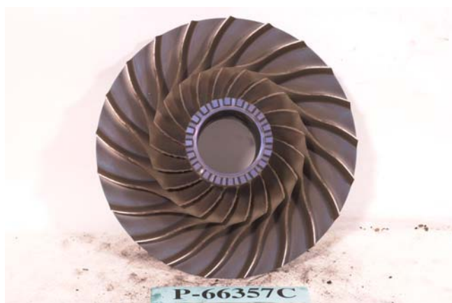
PHOTO 9: 2 ND -STAGE IMPELLER DAMAGE
