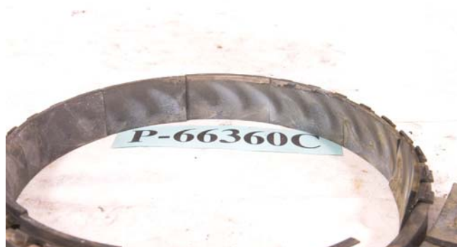
PHOTO 19: SCORED 1 ST -STAGE SHROUD SEGMENTS
