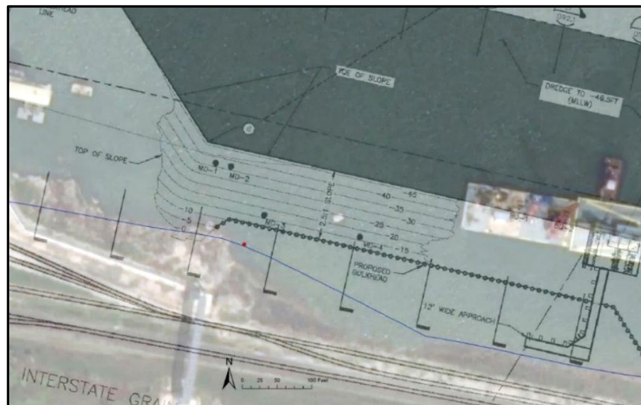
Figure 5. Excerpt of the June 23, 2020 Schneider Engineering revised dredging plan overlaid on Google Earth background, showing the TMI 2018 location of pipeline TX219 and the approximate accident location identified by a red dot. 11
