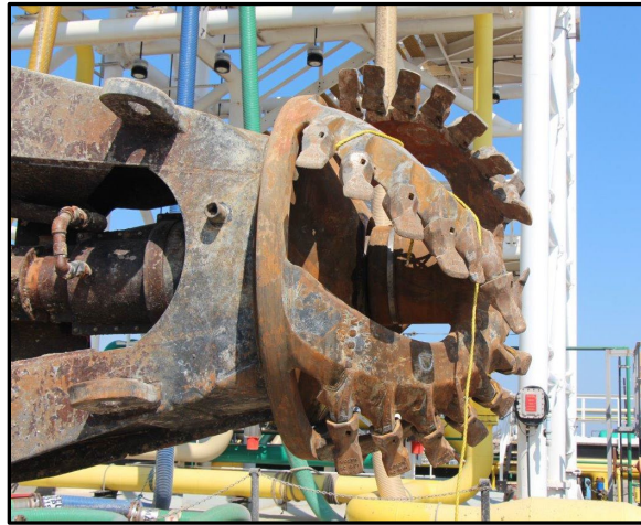
Figure 8. Post-accident photograph of the dredge Waymon Boyd cutterhead, September 17, 2020, courtesy U.S. Coast Guard.
