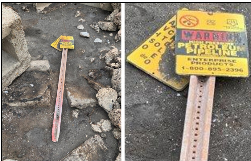
Figure 22. Downed permanent pipeline marker (GPS 2281-2282) near the accident location, September 14, 2020, U.S. Coast Guard photo.
