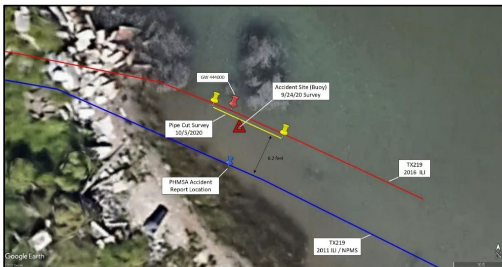
Figure 28. Annotated Google Earth base image showing approximate location data for pipeline TX219, including from south to north, the Rosen Group 2011 ILI inline inspection GPS location coordinates file (blue line), the SAM October 5, 2020 evidence recovery pipe cut survey (yellow markers), and the Rosen Group 2016 inline inspection GPS location coordinates (red line). The accident site as determined by a September 24, 2020 SAM survey of a buoy marker is indicated by a red triangle. The base imagery date is January 31, 2020.
