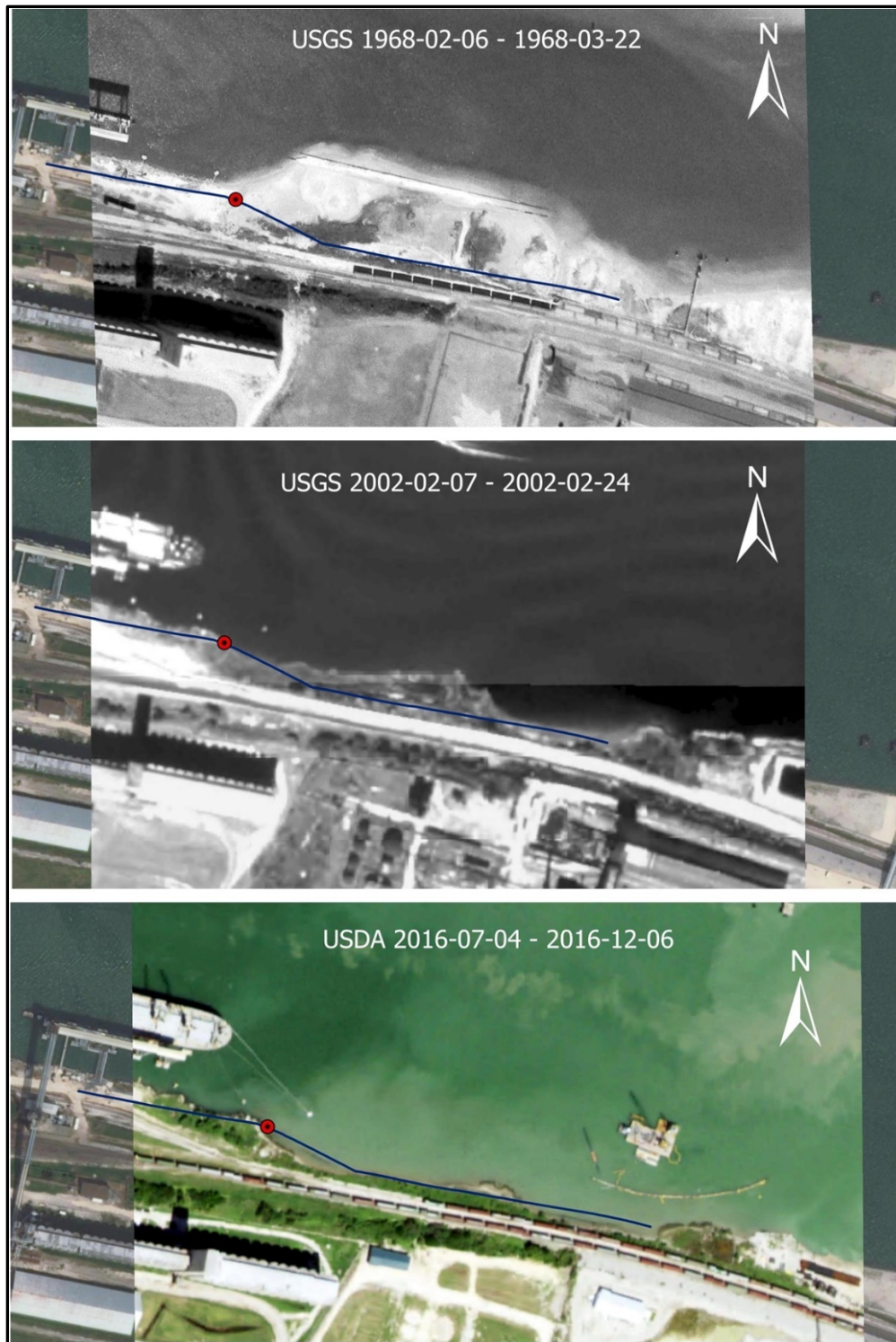
Figure 12, EPIC East Dock project area, 1968 (year the pipeline was installed), 2002, and 2016, showing the extent of land loss since its construction. USDA and USGS photographs overlaid on Google Earth image. The blue line indicates the location of pipeline TX219 (TMI Solutions, 2018) and the approximate accident location is indicated by the red circle.
