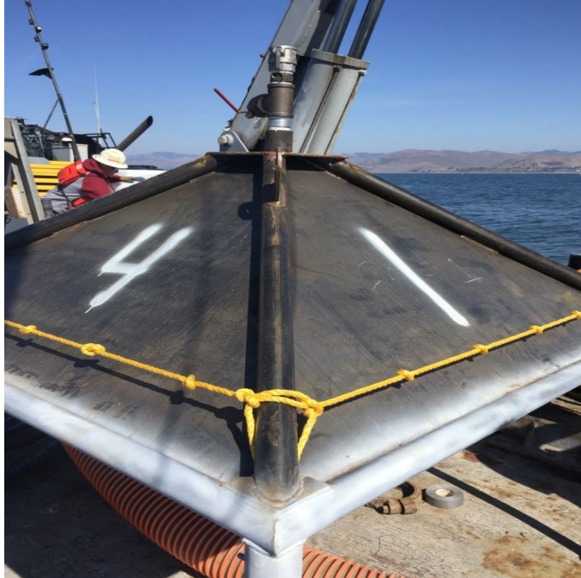
Figure 19. Pollution Dome Design and Fabricated and Ready for placement with a 53 Barrel Capacity. Photograph by Beta Offshore.
