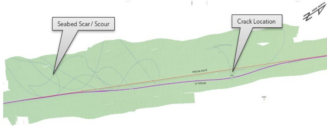
Figure 17. San Pedro Bay Pipeline original location and displacement. Scarring is noted by the dotted line in this graphic. Graphic by Beta Offshore.
