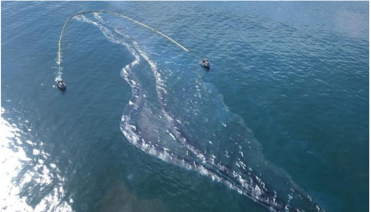
Figure 9. The unified command responded to and cleaned the crude oil spill off the California coast. Oil spill removal organization (OSROs) are shown towing skirted oil boom to contain the oil spill. Oct. 3, 2021. Photograph by U.S. Coast Guard.
