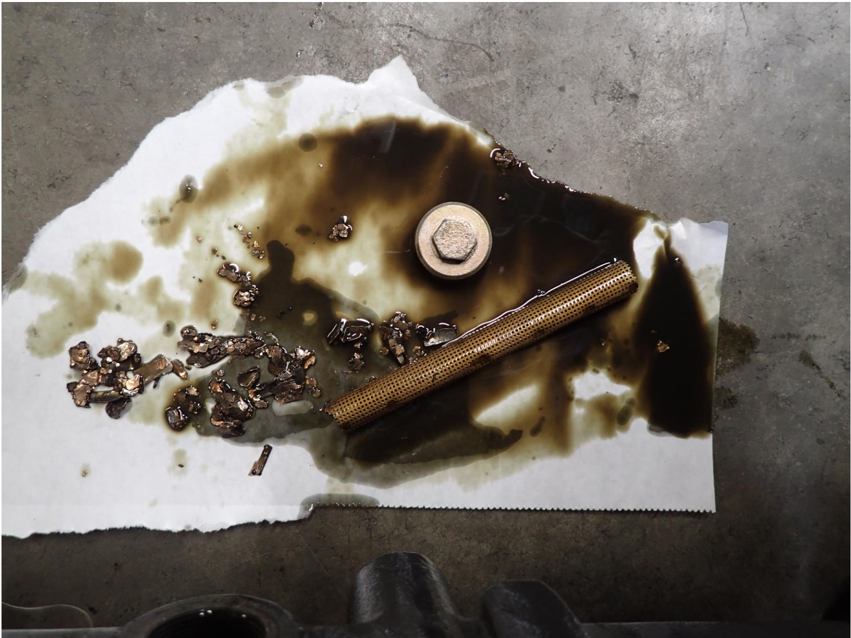
Photo 4 – Oil filter debris (Photo courtesy of the NTSB)
