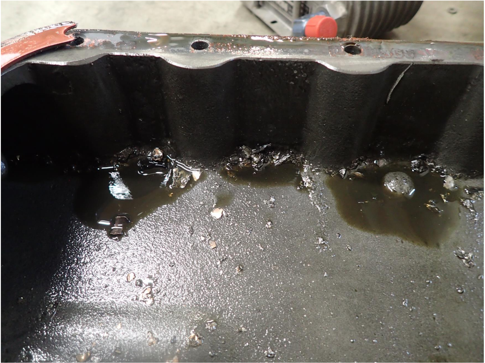
Photo 2 – Metal shavings in oil pan (Photo courtesy of the NTSB)
