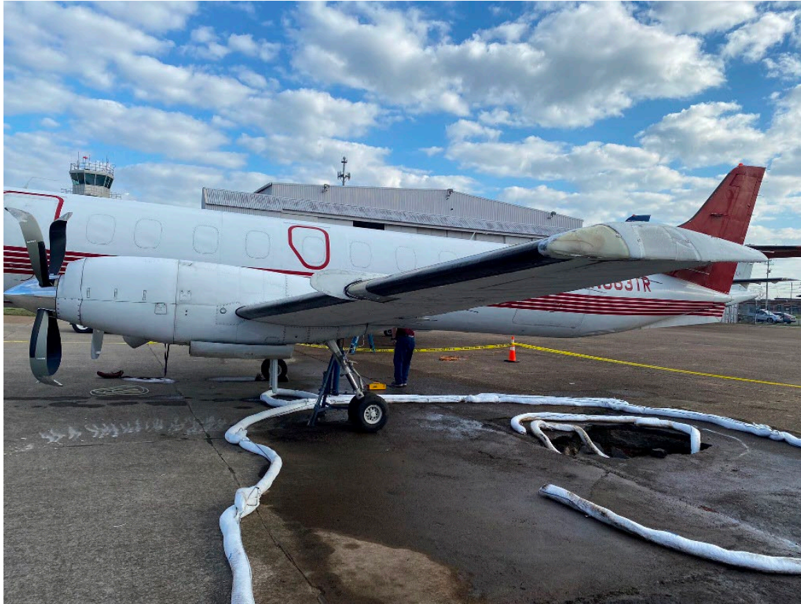
Photograph 2 - View of LH Side of Airplane and Damage to MLG and Propeller (Courtesy of FAA)
