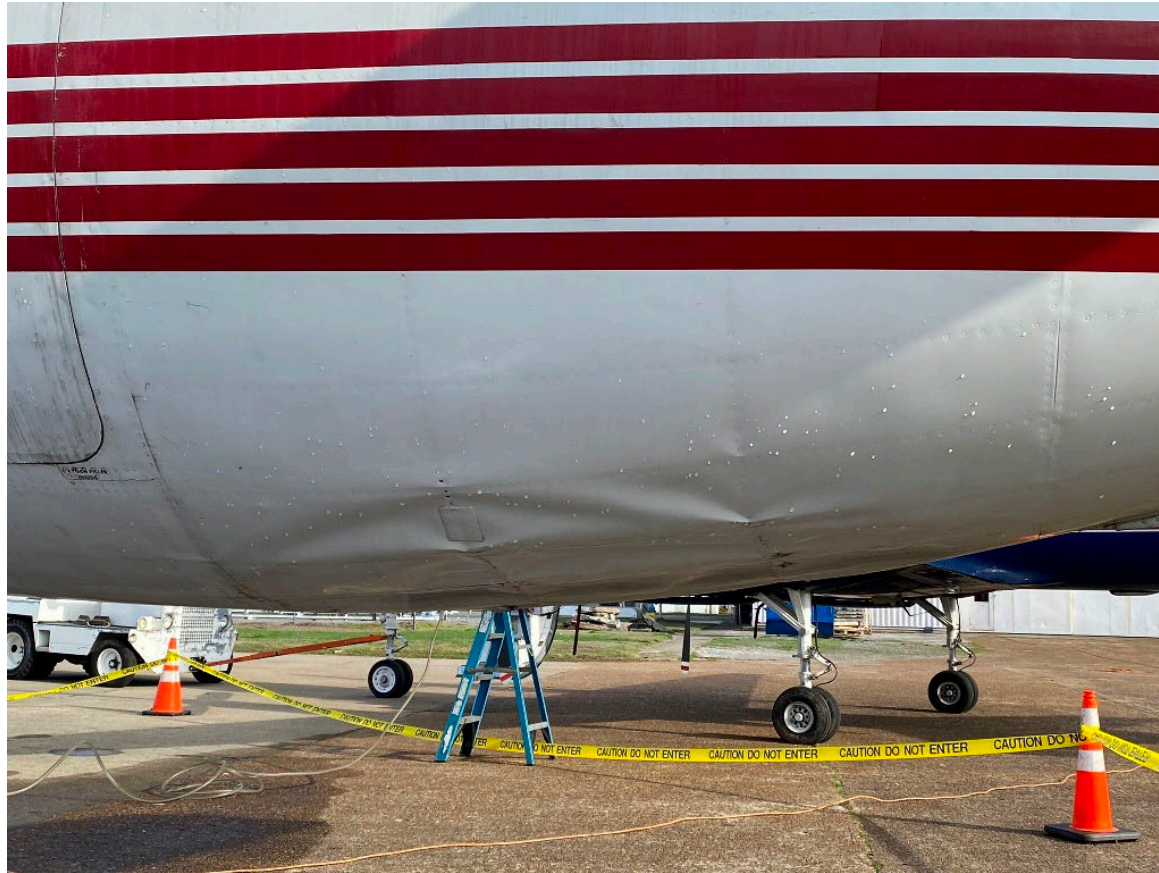
Photograph 3 - Damage of Lower Fuselage (Courtesy of FAA)
