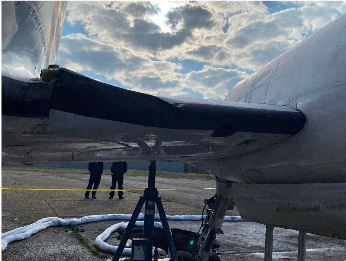
Photograph 4 - Damage to LH Wing Root (Courtesy of FAA)
