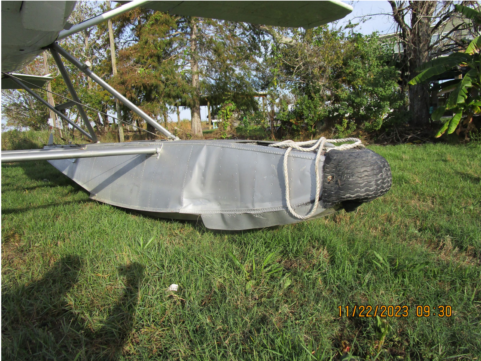
Photograph 3 - Damage to left float (Courtesy of FAA)
