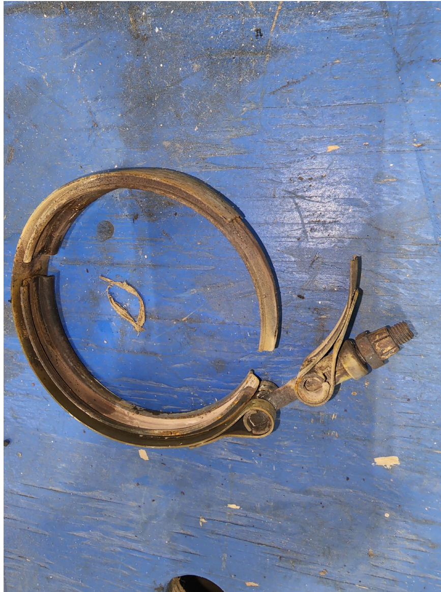
Photograph 3 - Fractured V-band clamp (Courtesy of FAA)
