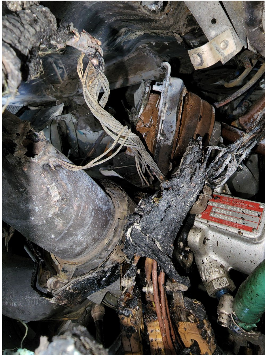
Photograph 4 - Engine accessory damage (Courtesy of FAA)
