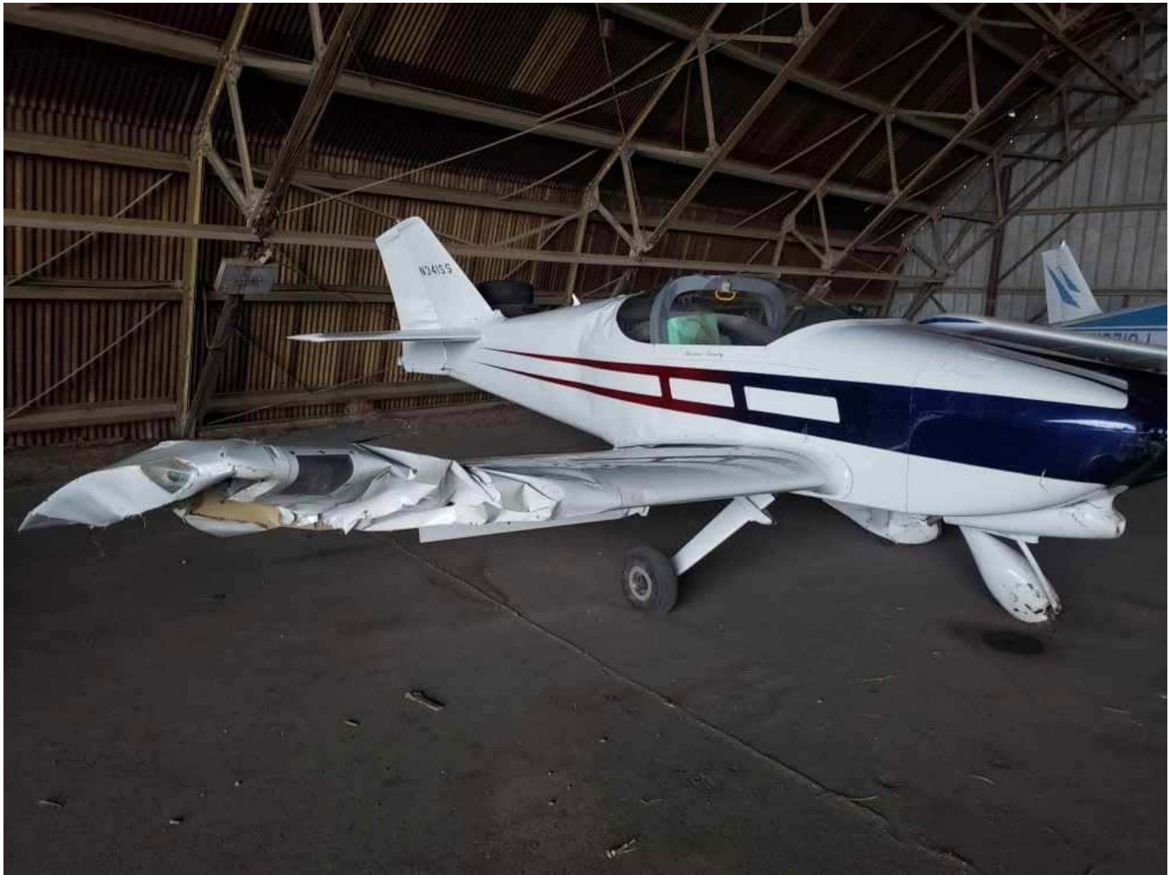
Photo 3 – Right view showing damage to the right wing, vertical stabilizer, and the rudder. Photo courtesy of the pilot.
