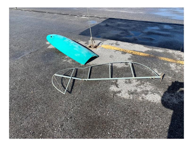
Photo 2 – View of the left wing tip and bent elevator. (Photo courtesy of the FAA)
