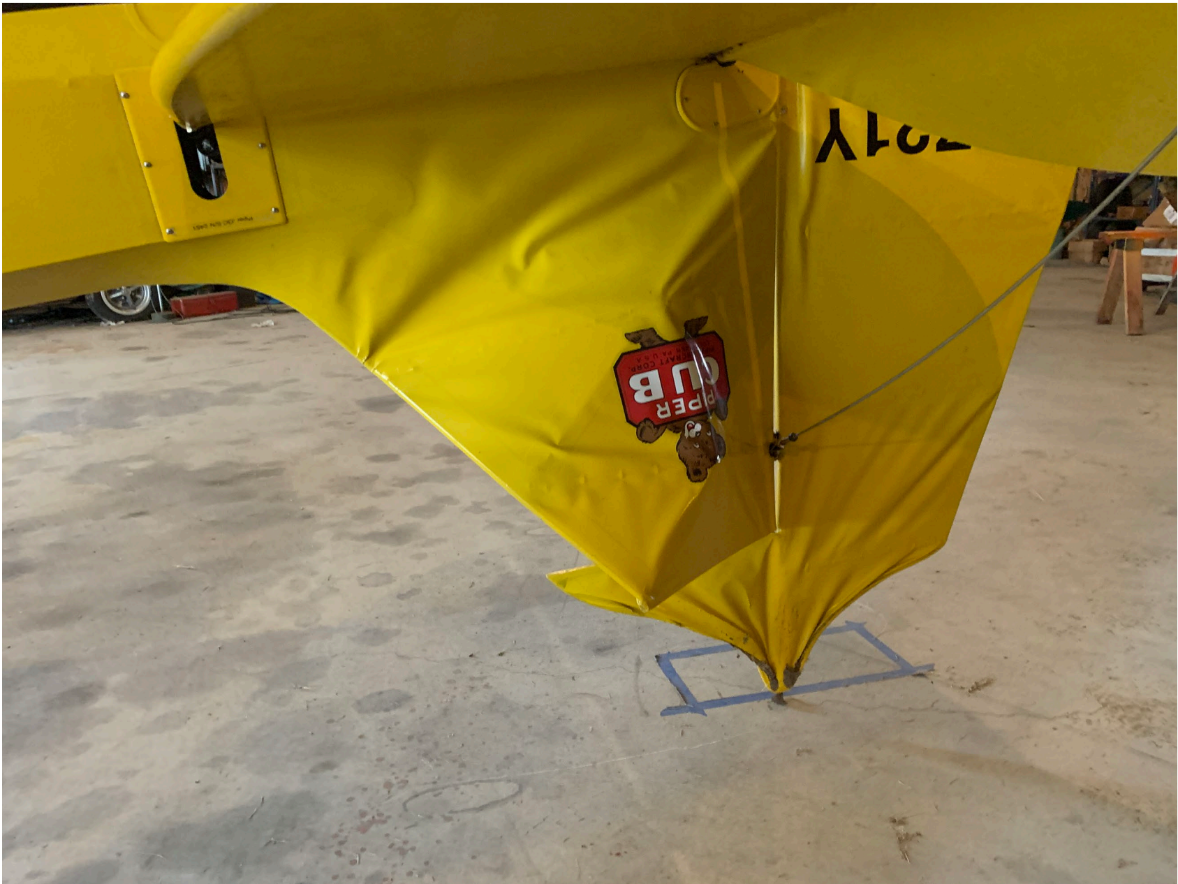
Photo 1 - Damaged Vertical Stabilizer, Courtesy of FAA
