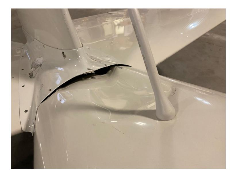
Photo 3 – View of the damage to the fuselage. (Photo courtesy of the FAA)
