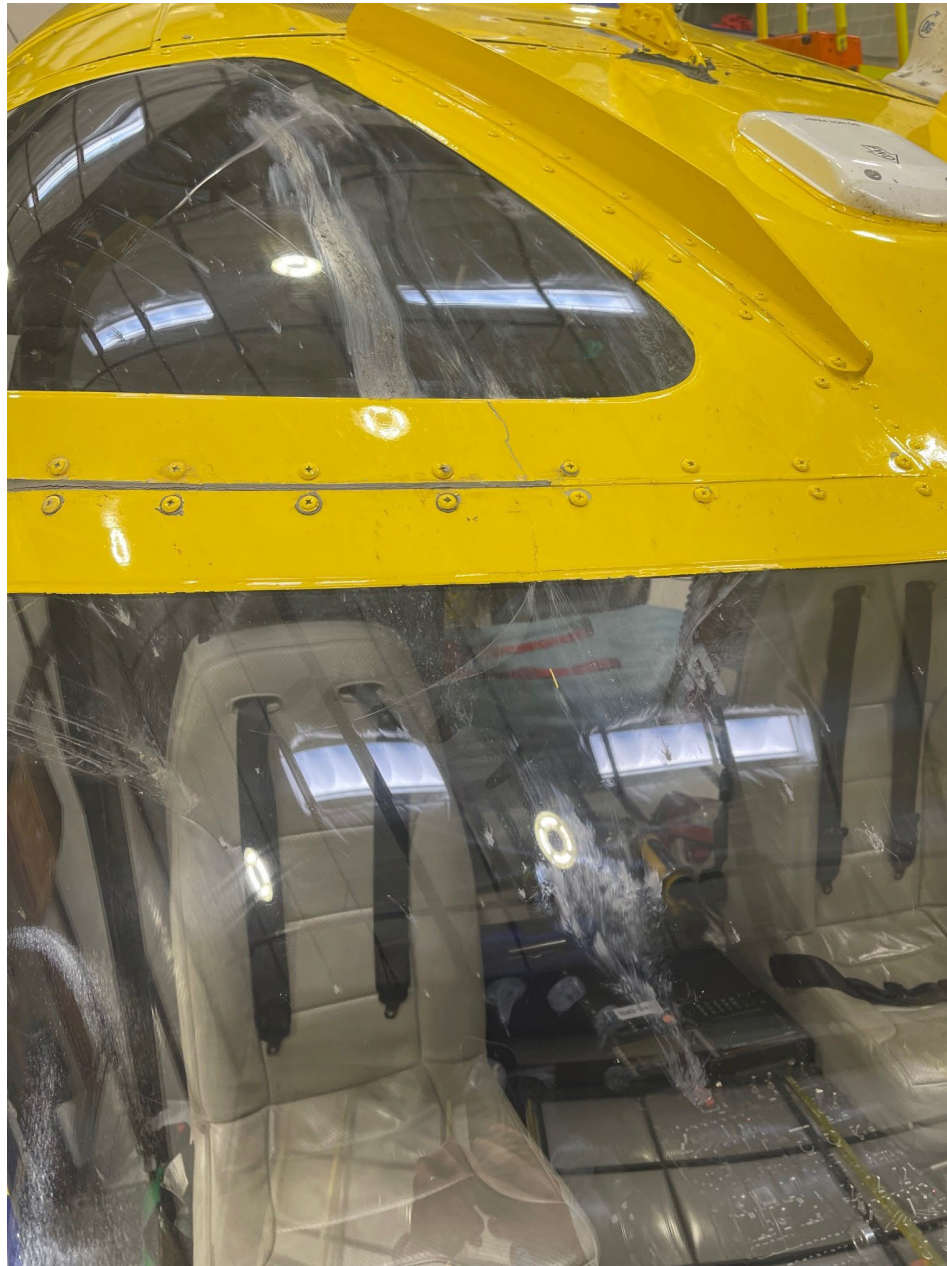
Photo 1 – Broken windshield support beam
