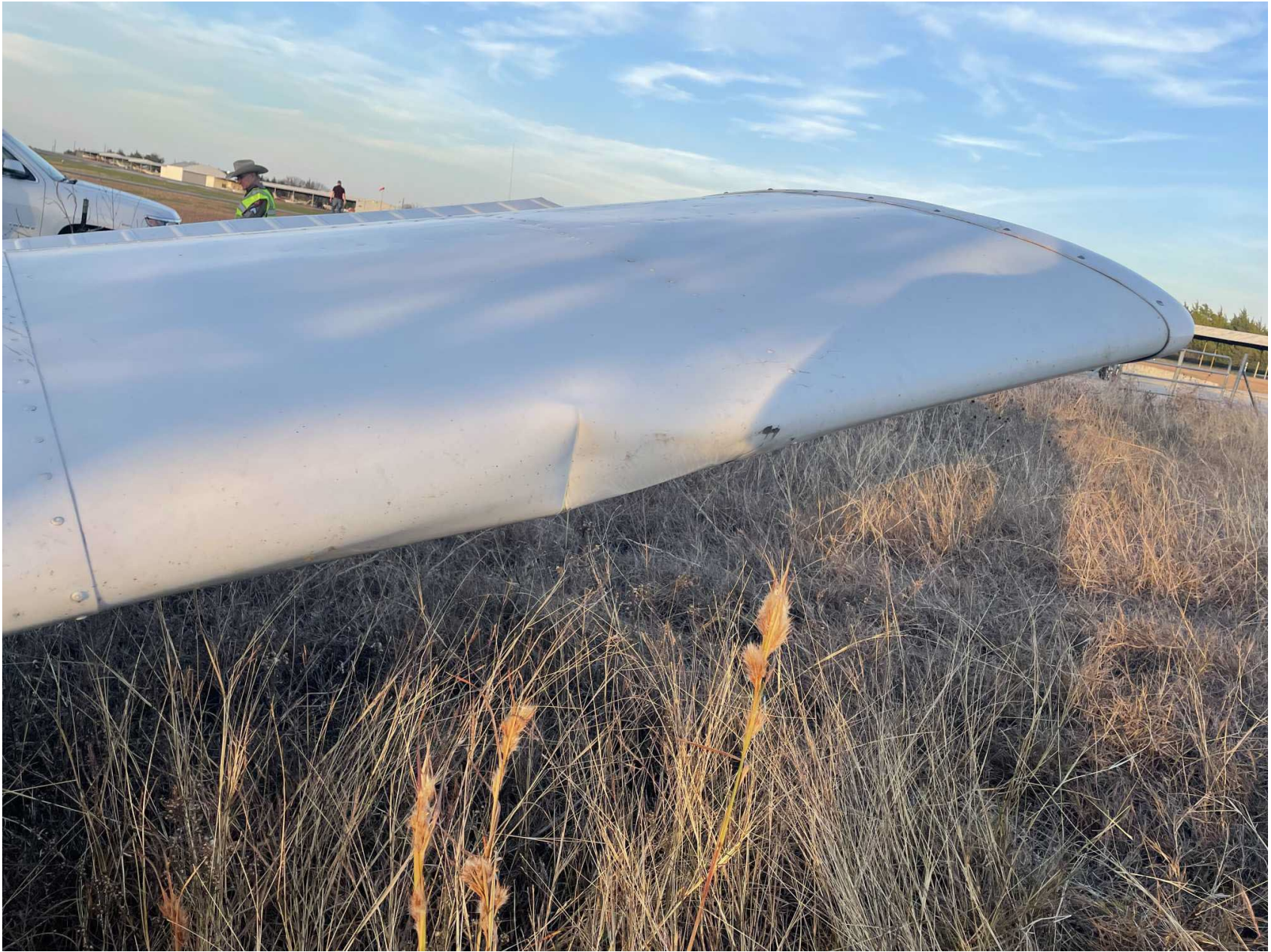
Photo 2 – Left Wing Damage, Photo Courtesy of FAA
