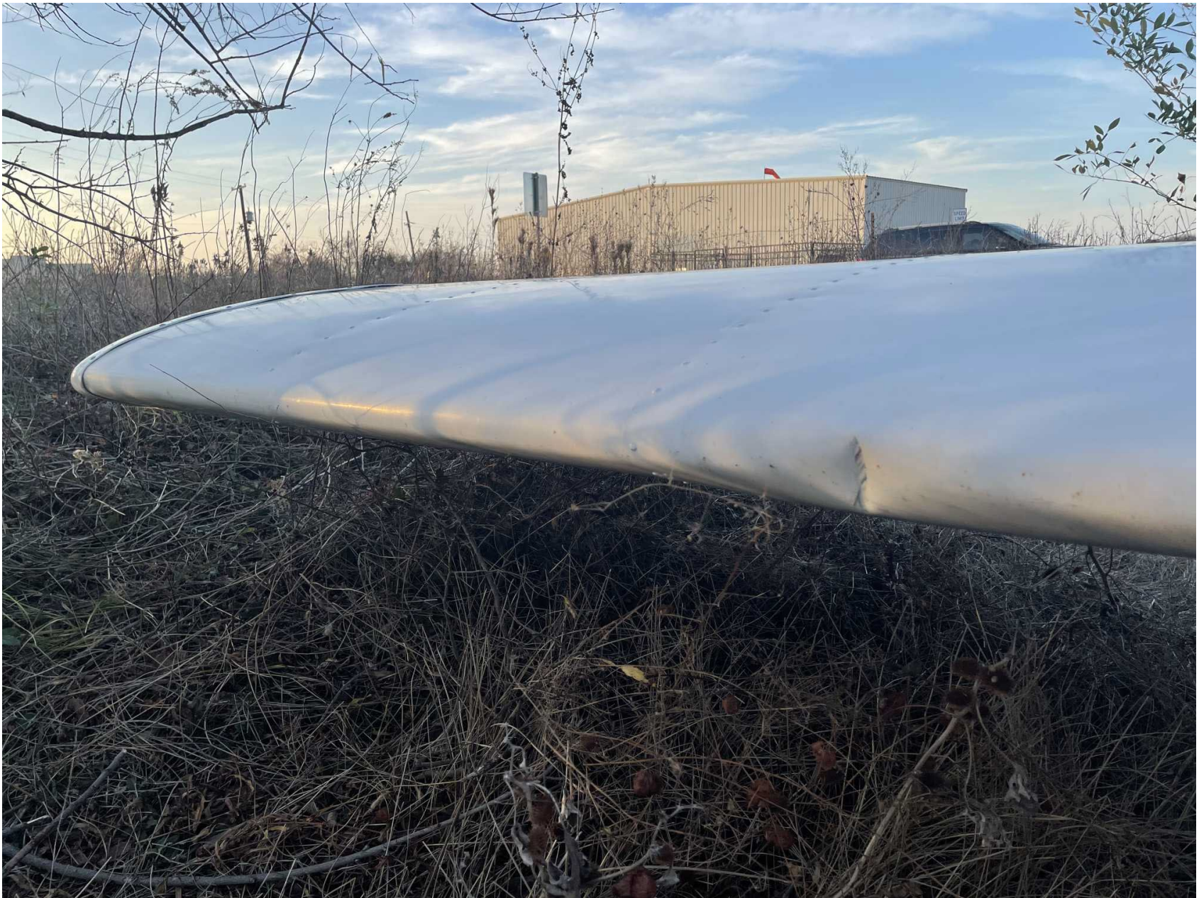
Photo 3 – Right Wing Damage, Photo Courtesy of FAA
