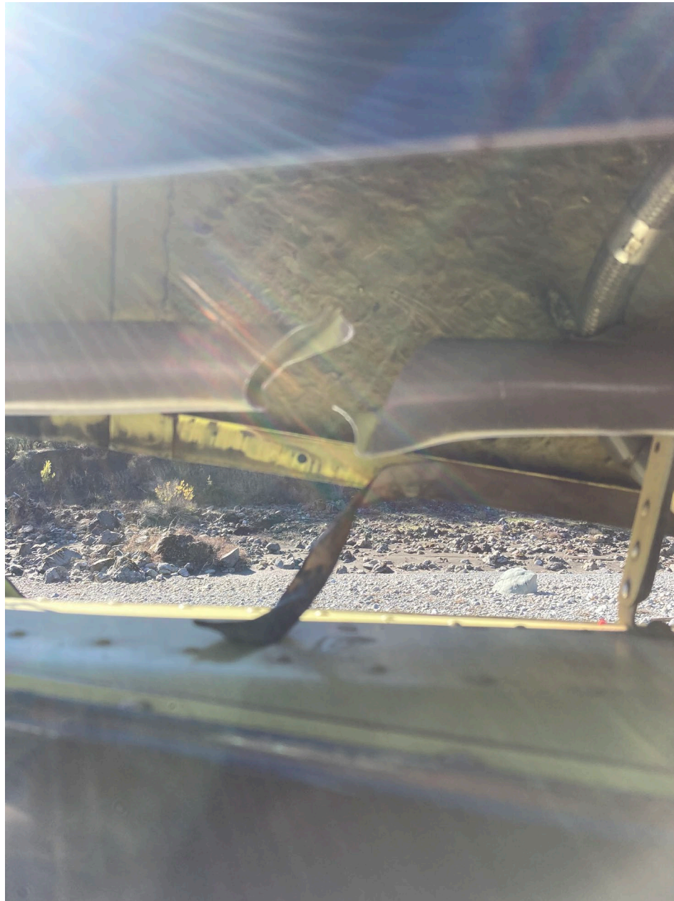
Photo 1 – Separated Tail Rotor Drive Shaft (Photo Courtesy of Pilot)
