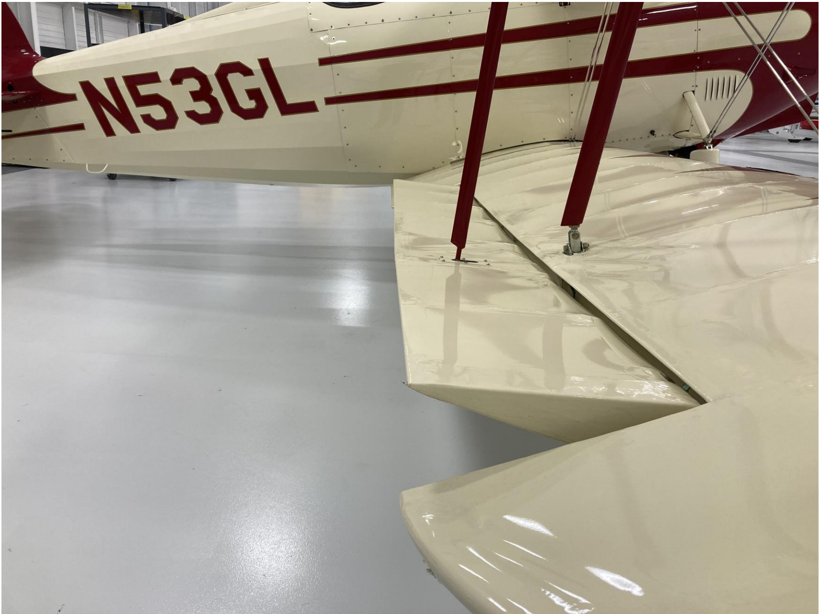
Photo 1 – Damage to the right wing and aileron (Courtesy of CFI)
