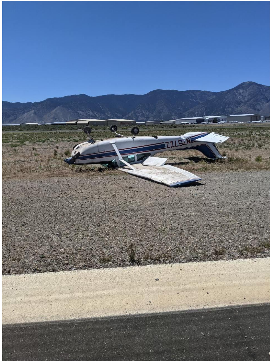
Photo 1 – View of the inverted airplane with damage to the right wing lift strut and empennage (Courtesy of FAA)
