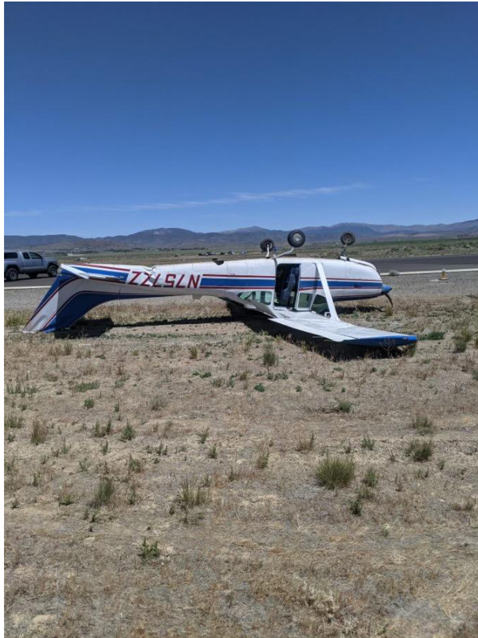
Photo 2 – View of the inverted airplane with damage to the empennage (Courtesy of FAA)
