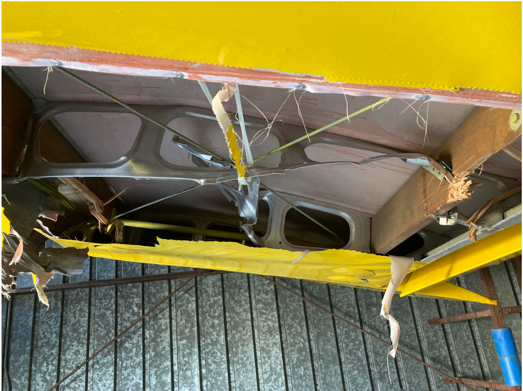
Photo 2 – Right wing internal damage
