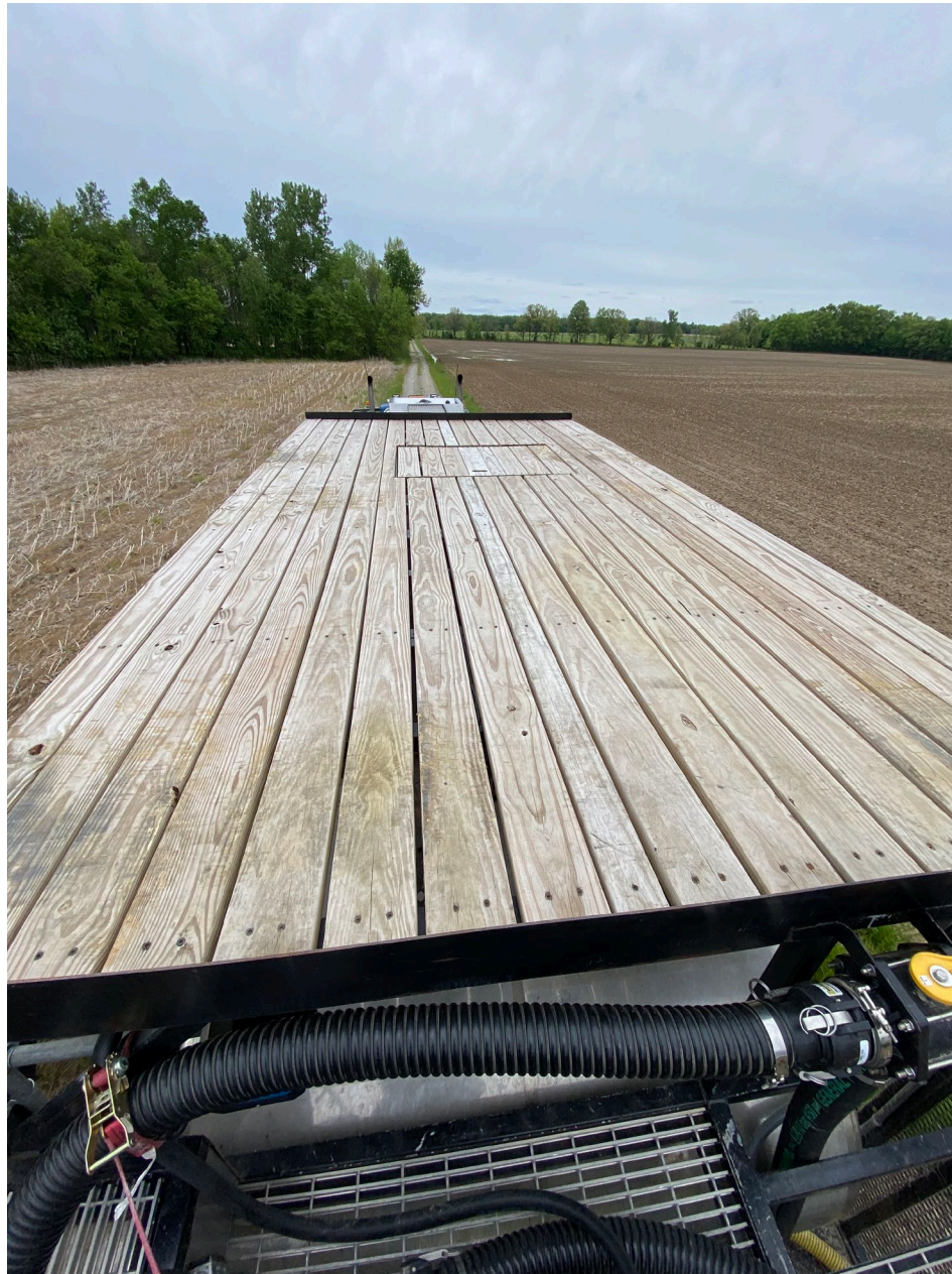
Photo 4 – Landing pad on truck. Courtesy of FAA
