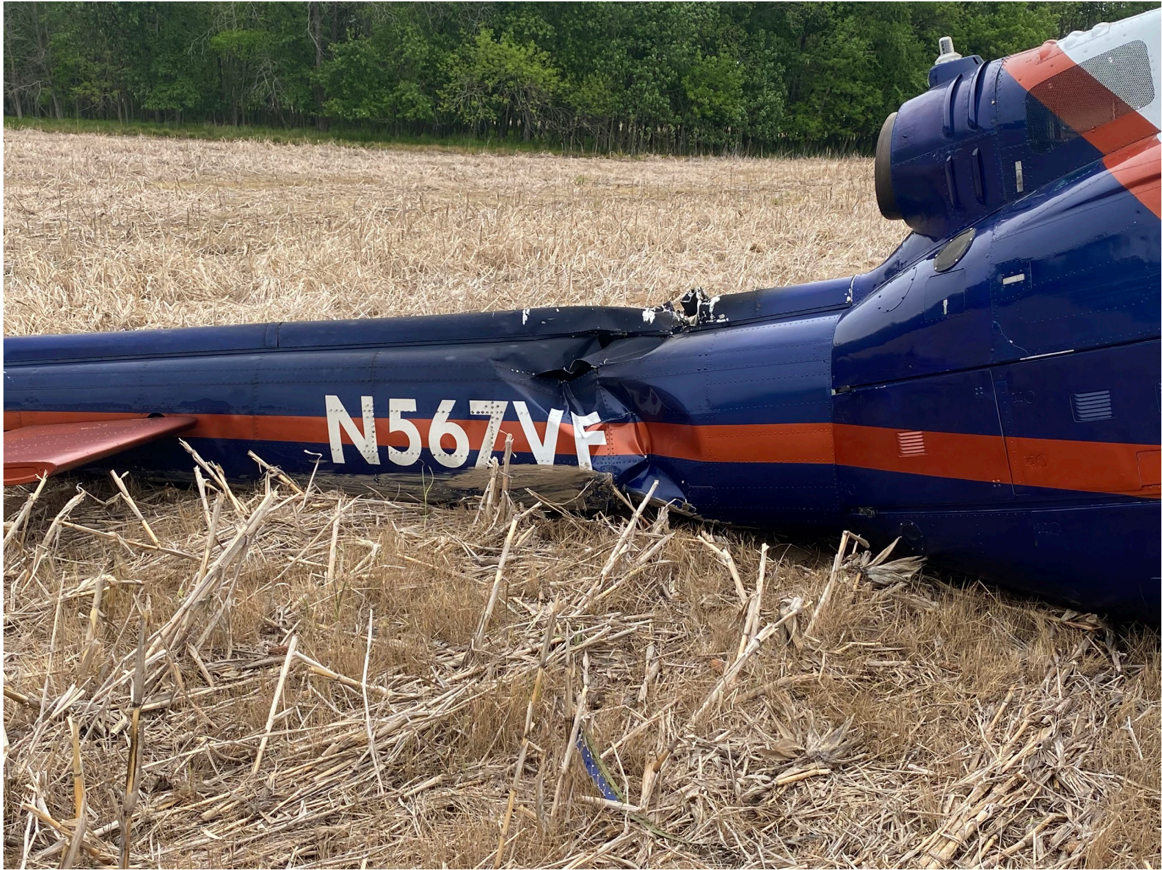
Photo 2 – Fuselage damage. Courtesy of FAA
