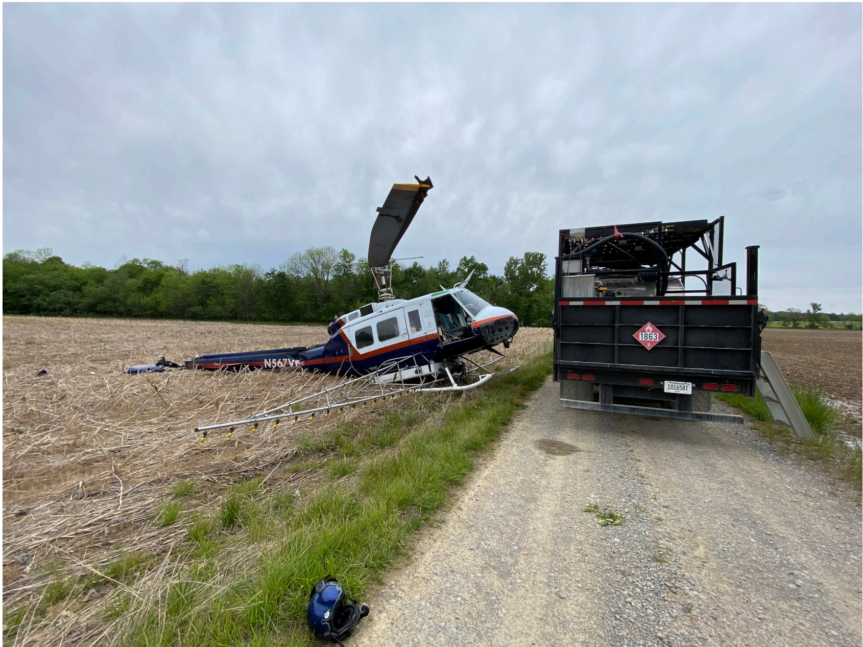
Photo 1 – Helicopter after tipping of truck landing pad. Courtesy of FAA
