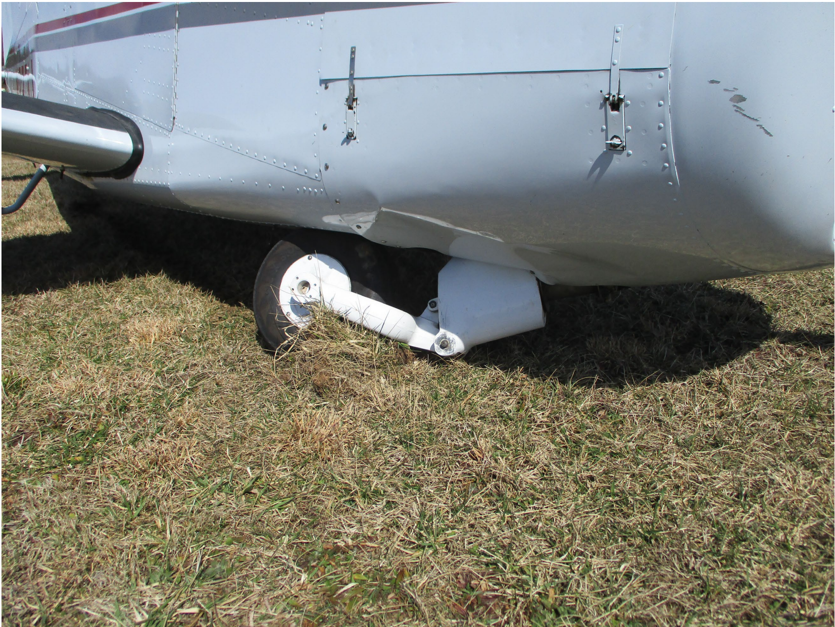
Photo 2 – View of collapsed nose landing gear. (Photo courtesy of FAA)
