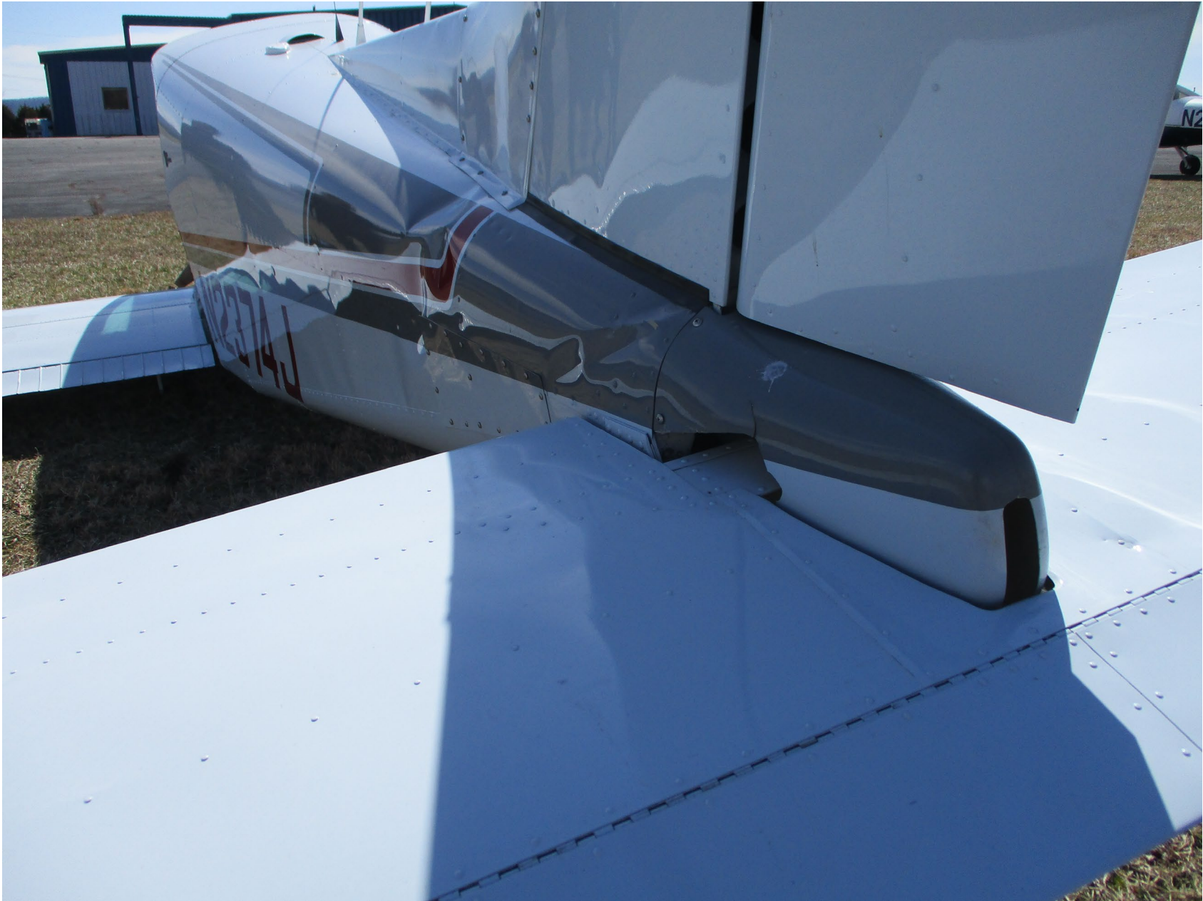
Photo 3 – View of the damage to the fuselage and empennage. (Photo courtesy of FAA)
