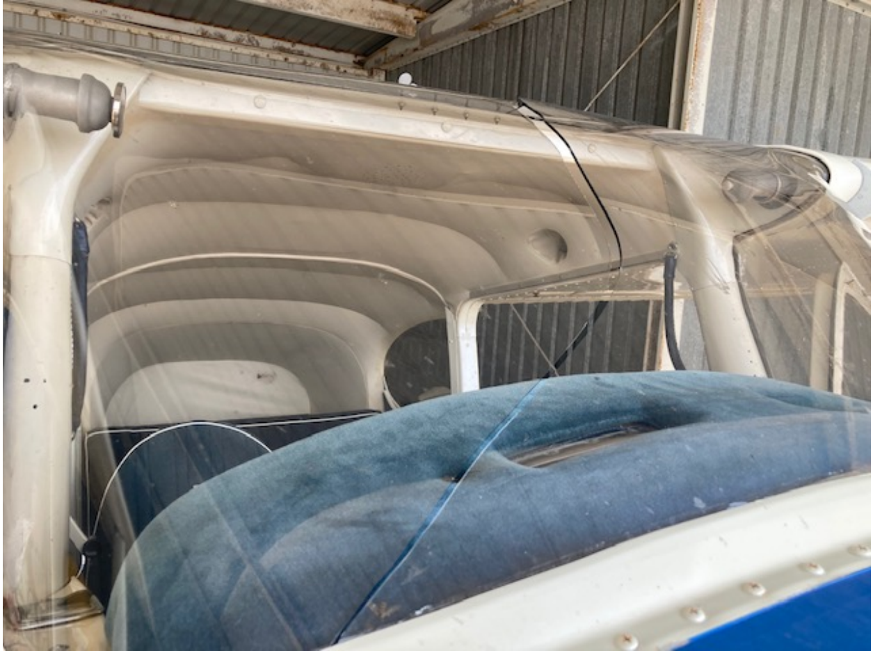
Photo 3: Damage to the Windshield
