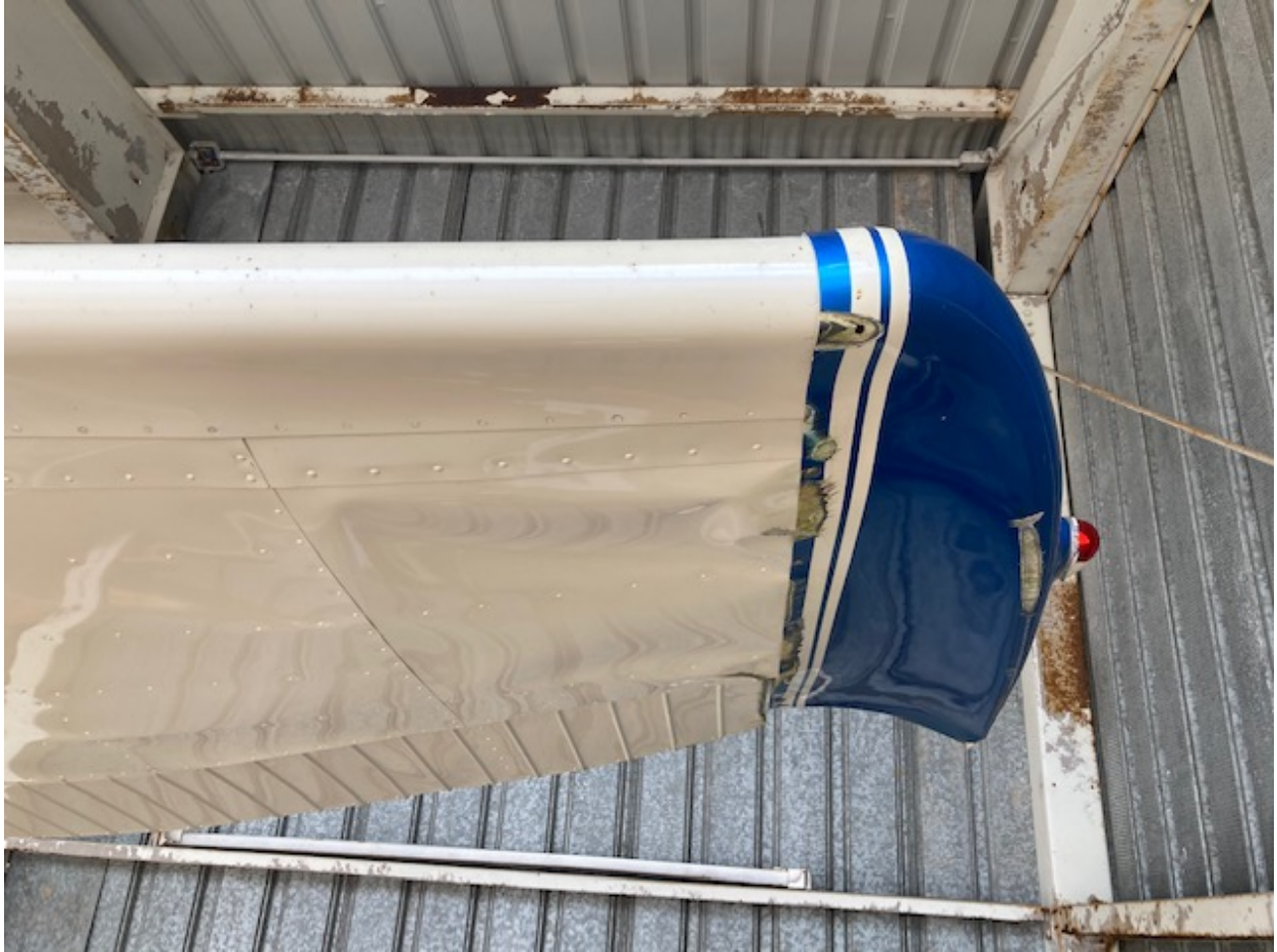
Photo 2: Damage to the Lower Surface of the Left Wing
