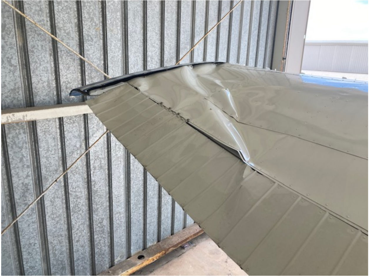
Photo 1: Damage to the Upper Surface of the Left Wing Damage
