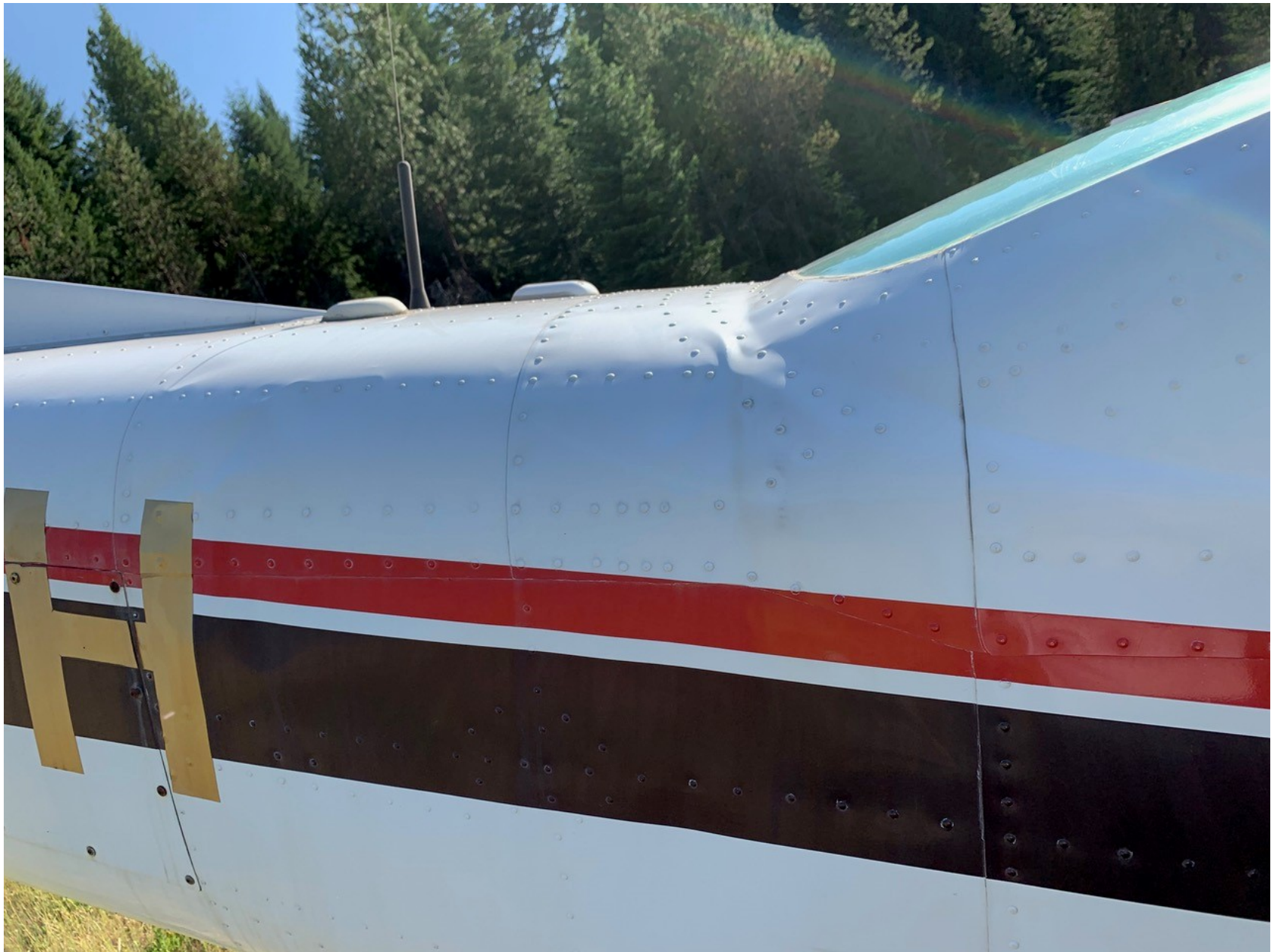
Photo 2 – View of damage to the aft fuselage (Courtesy of FAA)
