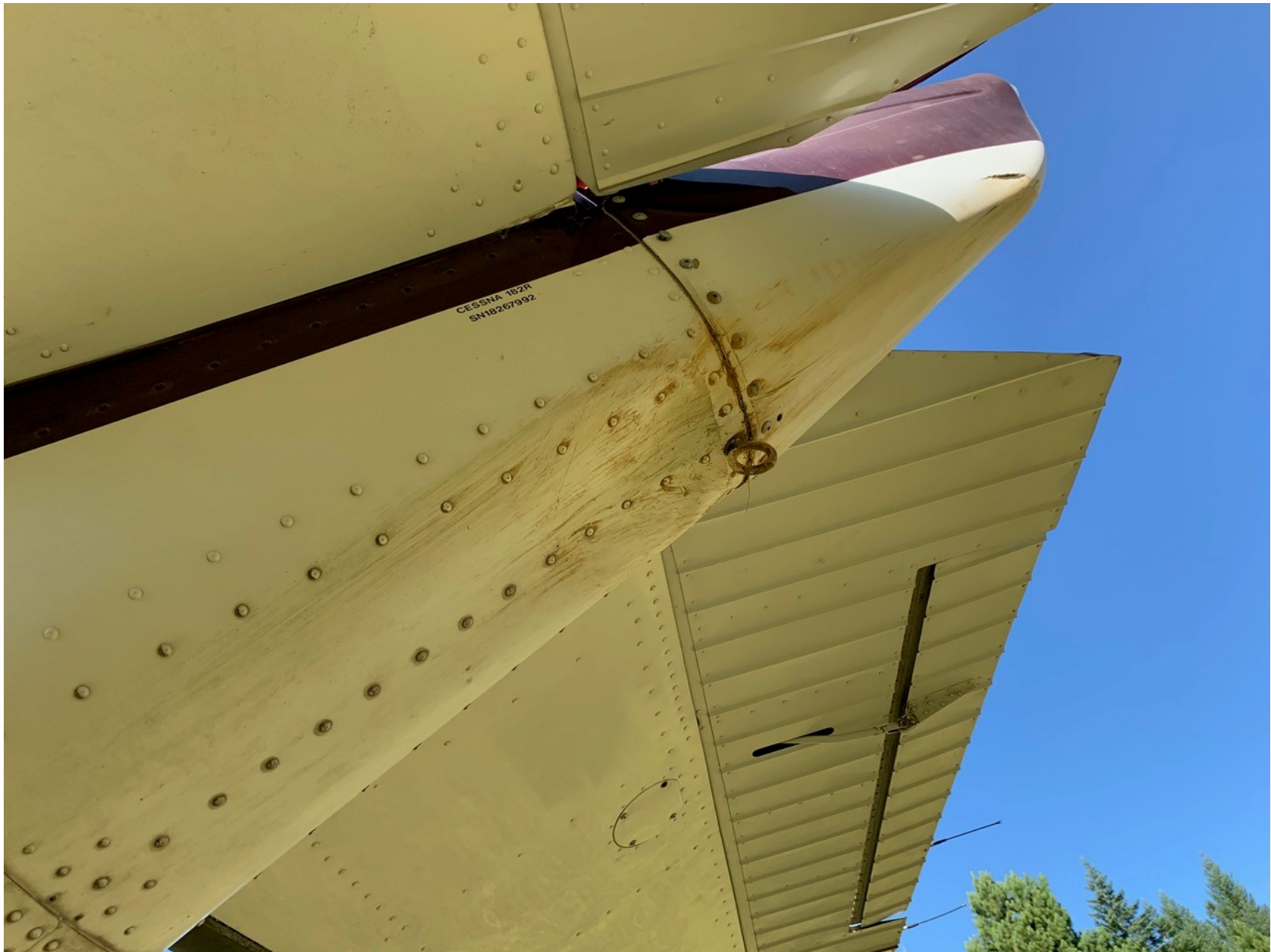
Photo 1 – View of damage to tail bulkhead and aft stringers (Courtesy of FAA)
