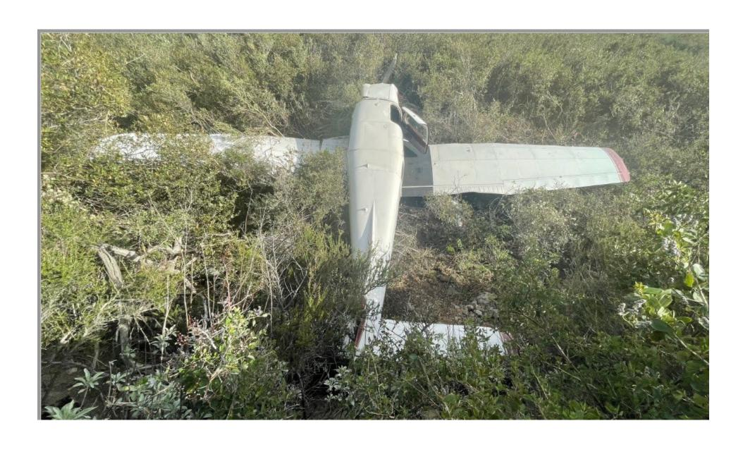
Photo 1-N42764, top view of airplane, showing damage to the wings. Photo courtesy of the pilot.
