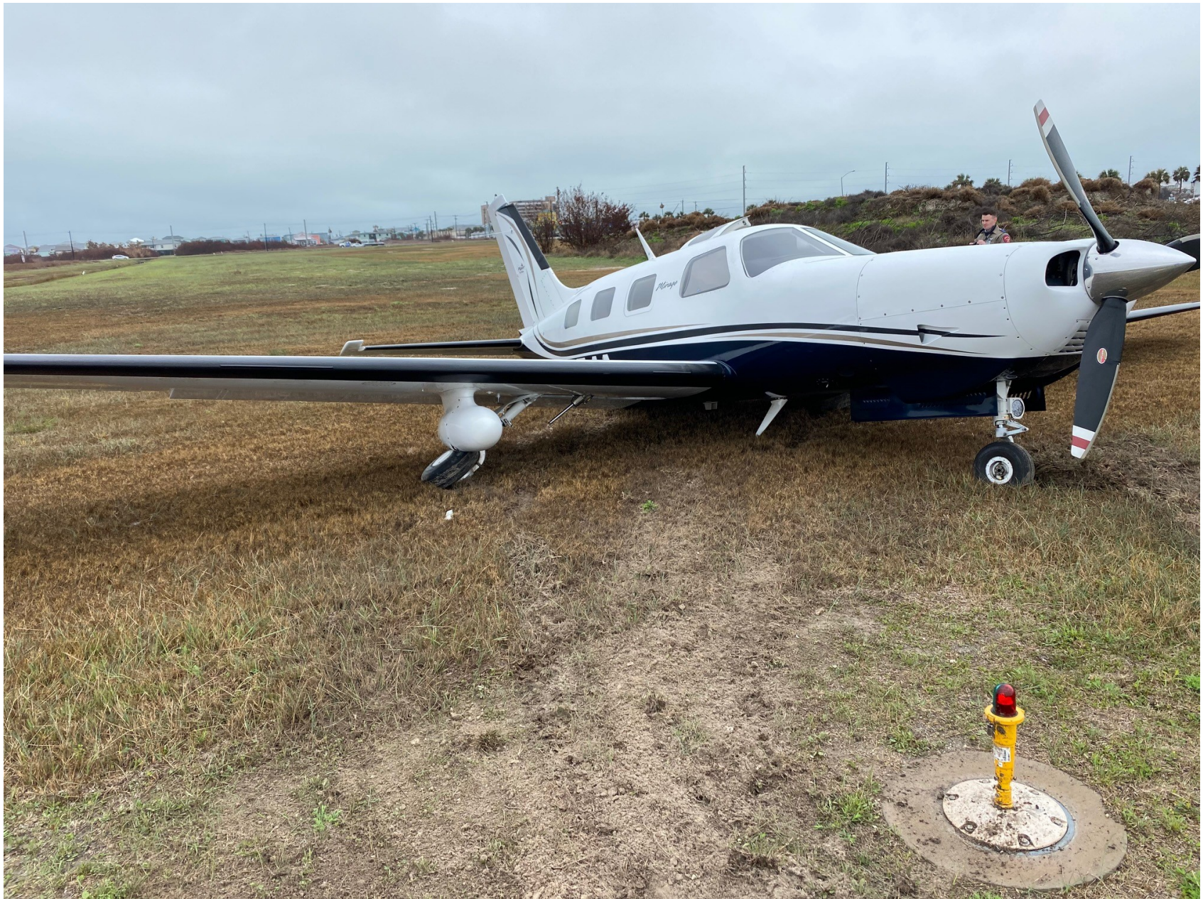
Photo 1 – Photograph of Airplane Sitting in Grass with Collapsed Right Gear
