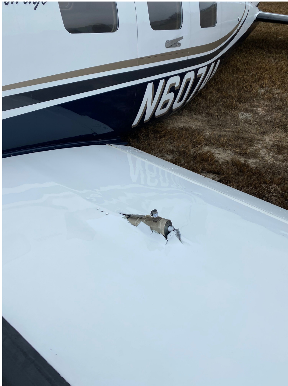
Photo 2 – Left-hand Landing Gear Actuator Protruding Though Left Wing
