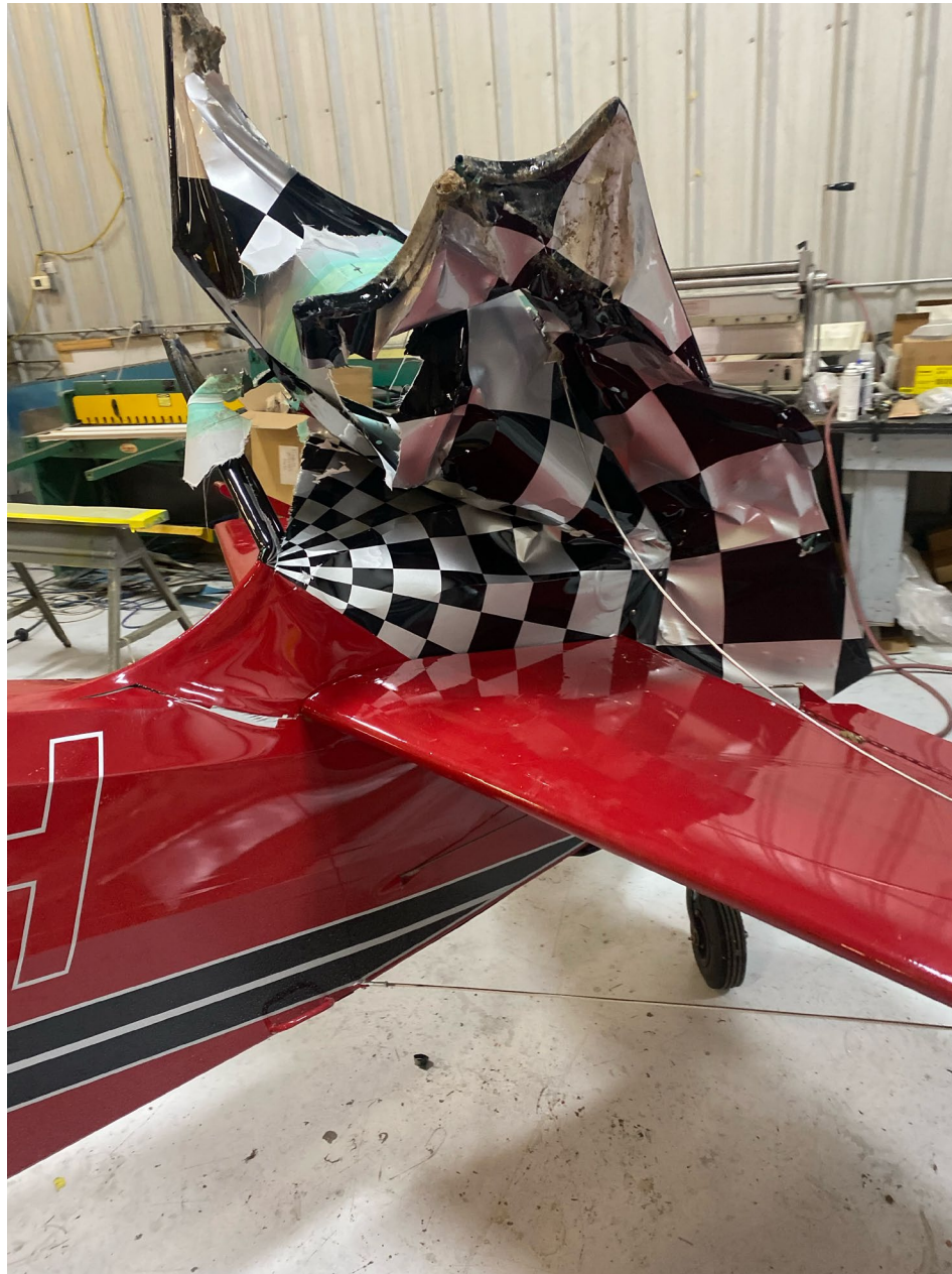
Photo 1 –N58BH, showing damage to the vertical stabilizer and rudder. Photo courtesy of the pilot.
