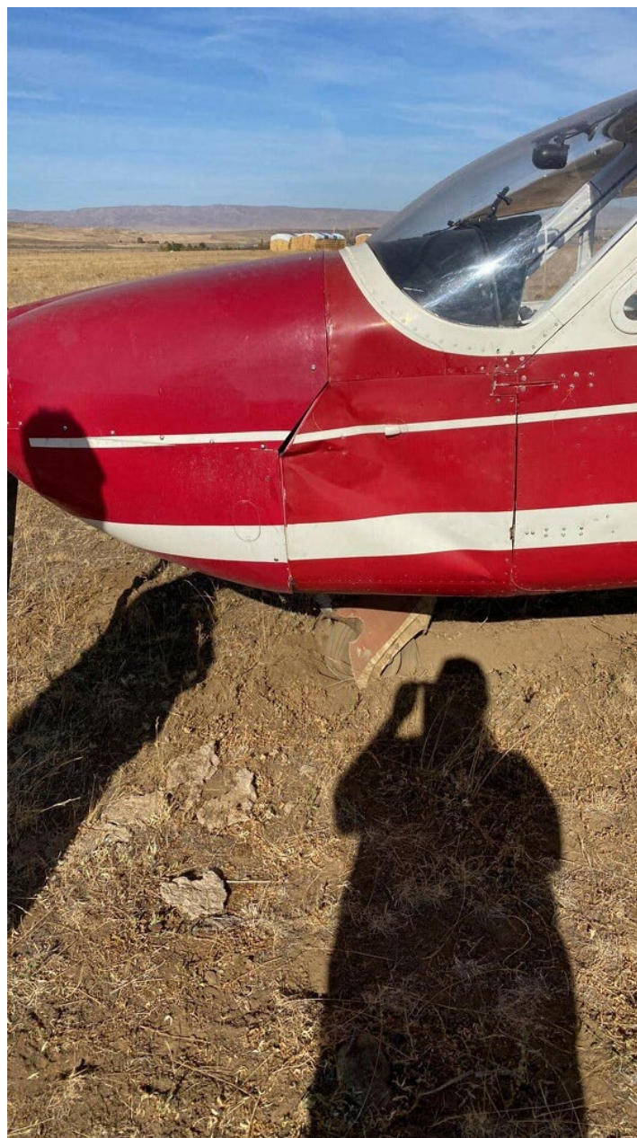
Photo 2 – Left-side view of N3388T, showing substantial damage to the fuselage. Photo courtesy of the pilot.
