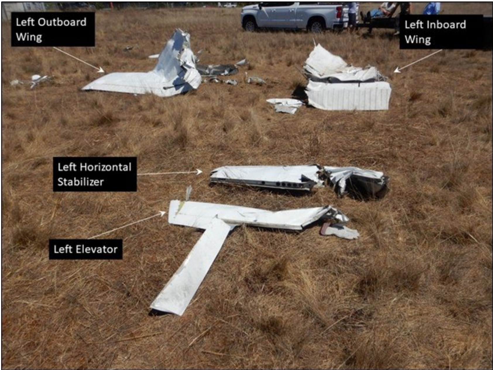
Photo 18 – Layout of the left wing, left horizontal stabilizer, and elevator
