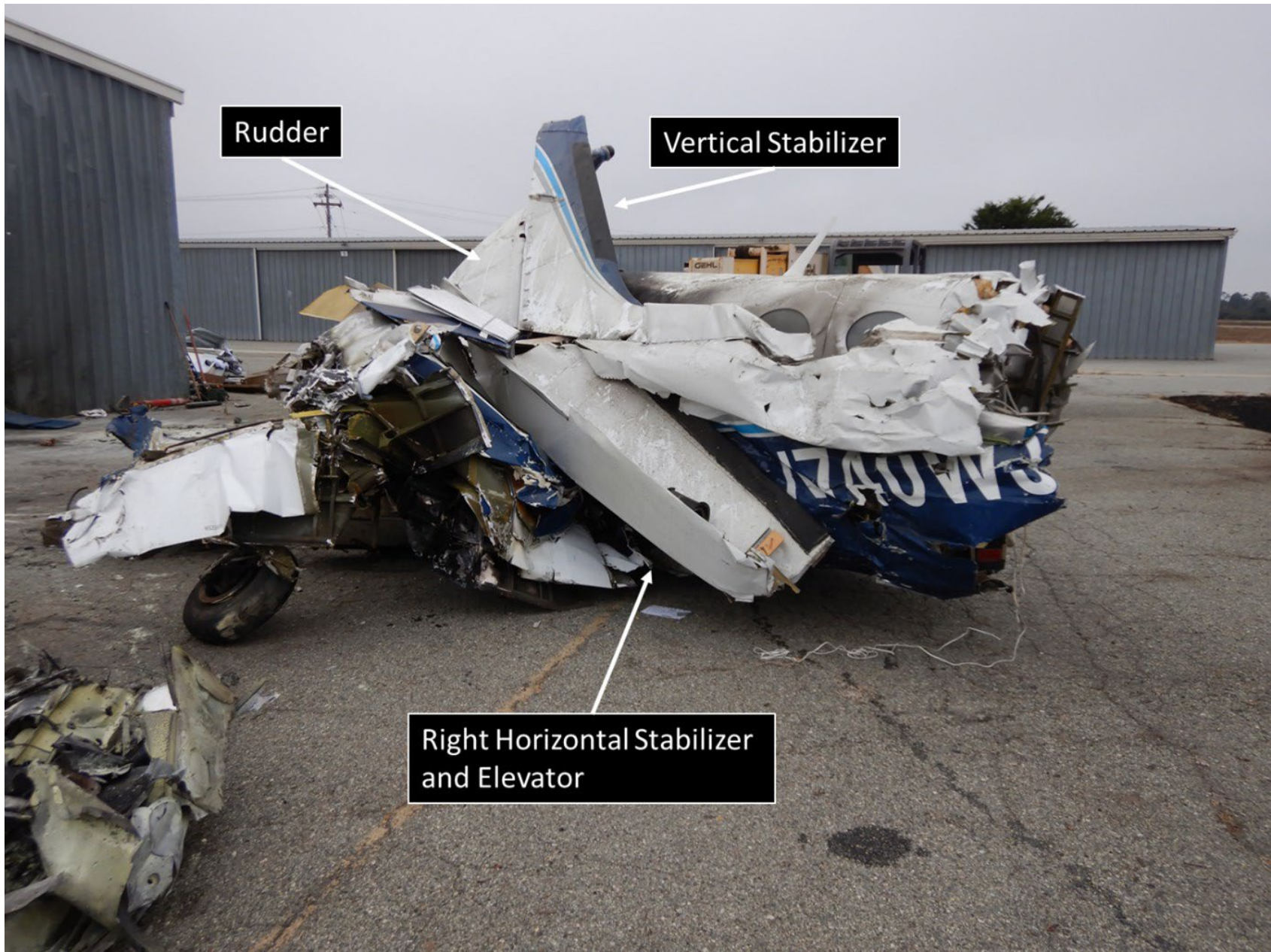
Photo 4 – N740WJ, left-side. The right side of the empennage is in view and wrapped around the left side of the fuselage.
