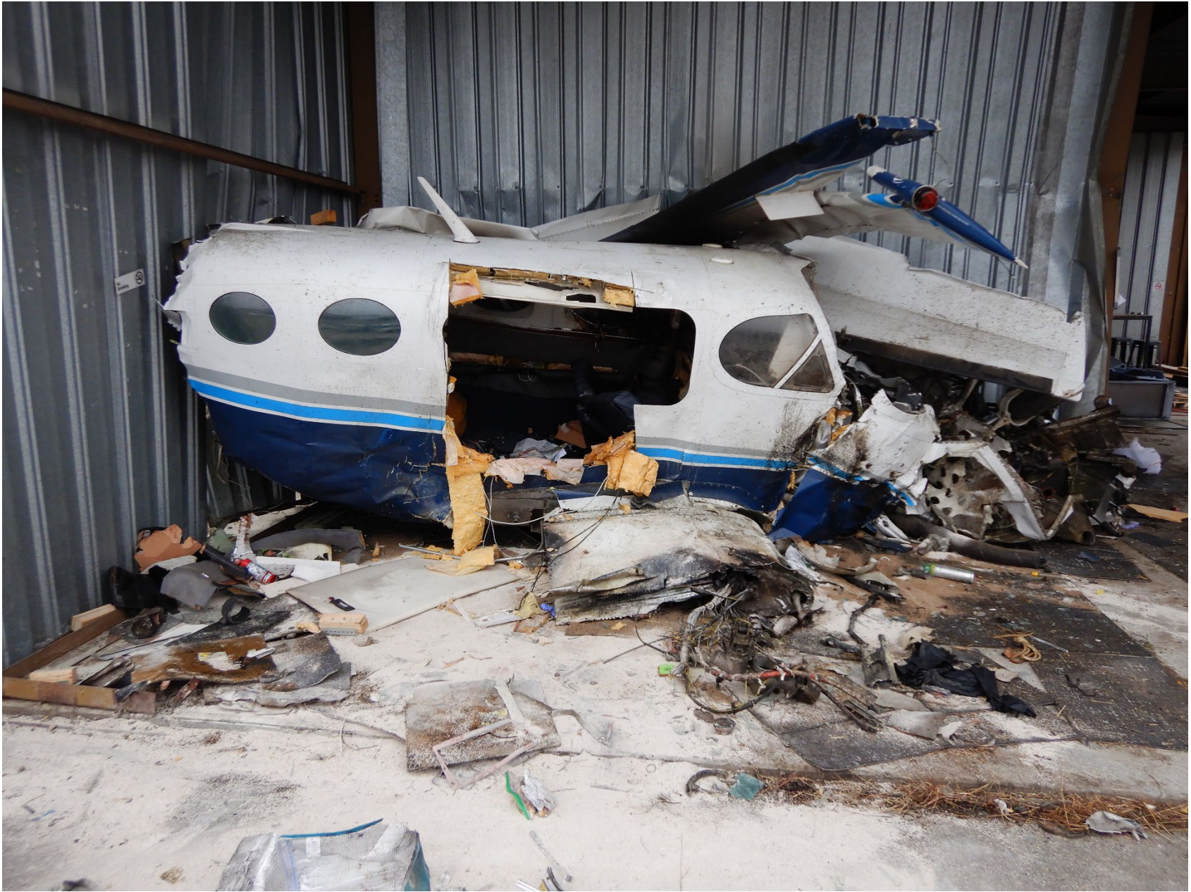
Photo 2 -N740WJ, showing the cutaway area used during recovery.
