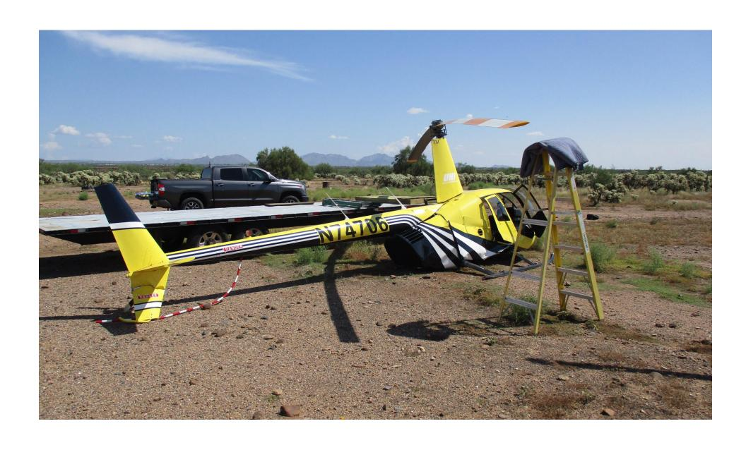
Photo 2-N74706, showing substantial damage to the lower vertical stabilizer. Photo courtesy of the FAA.
