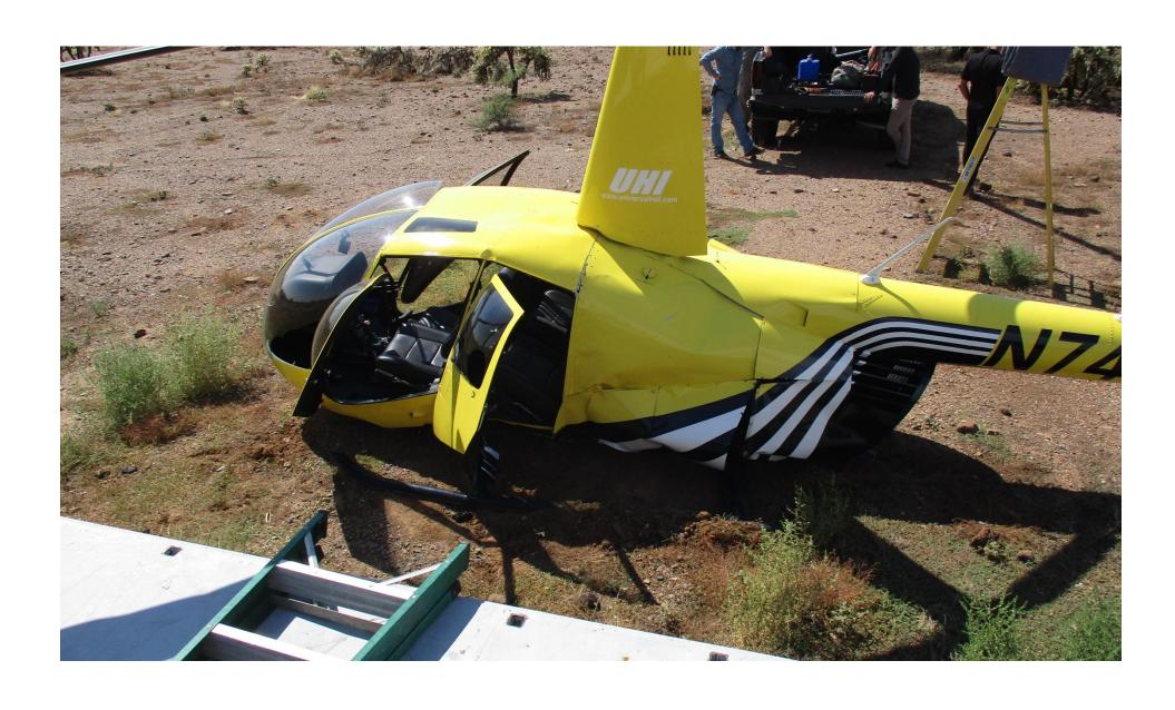
Photo 3 – N74706, showing substantial damage to the left side of the fuselage. Photo courtesy of the FAA.
