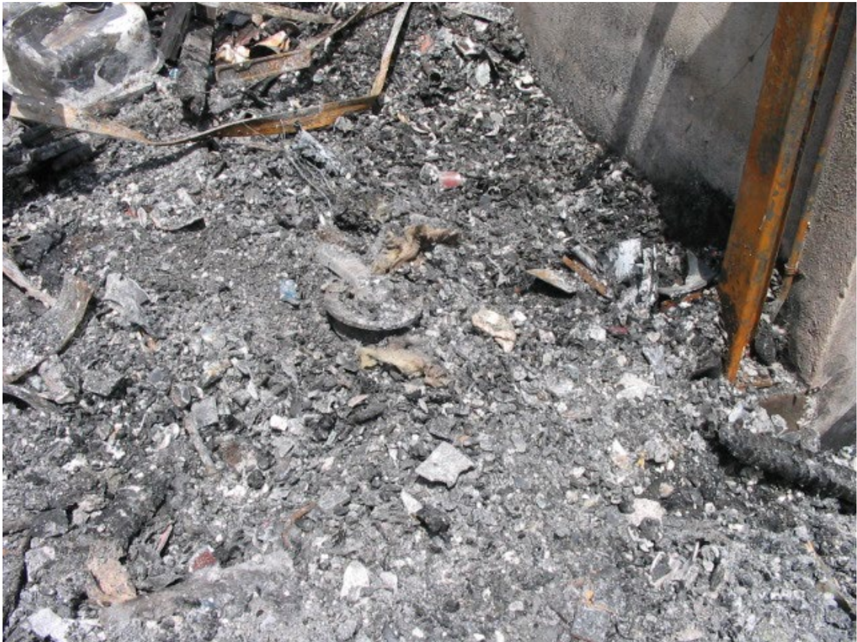
Photo 7 – Photo showing the left main landing gear and ash from the left wing. Photo courtesy of the FAA.
