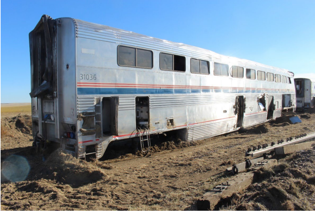
Figure 13 Photograph of the middle of the three uncoupled train cars. Coach Car ATK 31036 remained coupled to ATK 34077 in the lead and the Sleeper ATK 32007 that was trailing. Damage shown includes rescue damage caused by emergency responders and construction crews on scene. (Source: NTSB)
