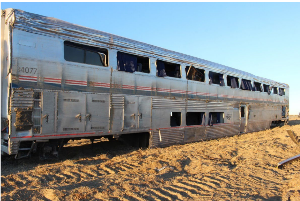
Figure 12 Photograph of westernmost uncoupled train car, ATK 34077, after the car had been righted. The Photograph shows the damage to the right side of the car caused by the contact with the ground. (Source: NTSB)
