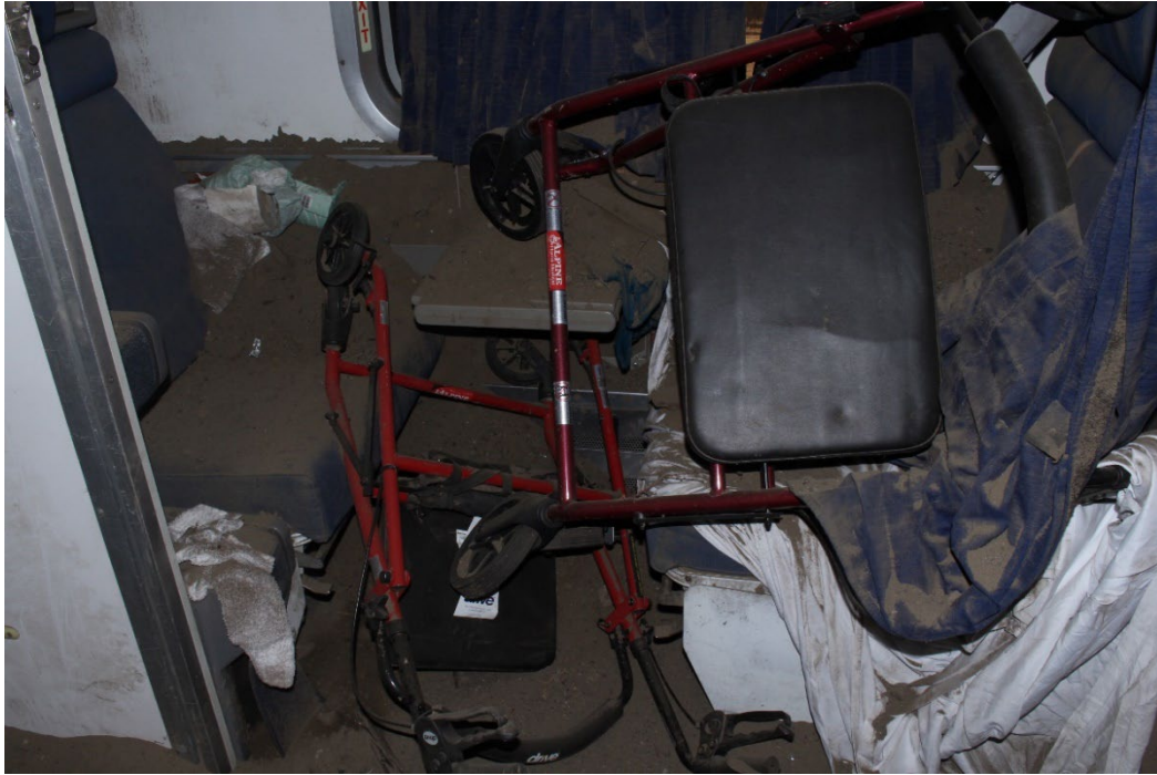
Figure 15 Photograph of the interior lower bedroom in Sleeper Car ATK 32007. The room is filled with dirt that infiltrated the car after the car window fell out of its frame. (Source: NTSB)
