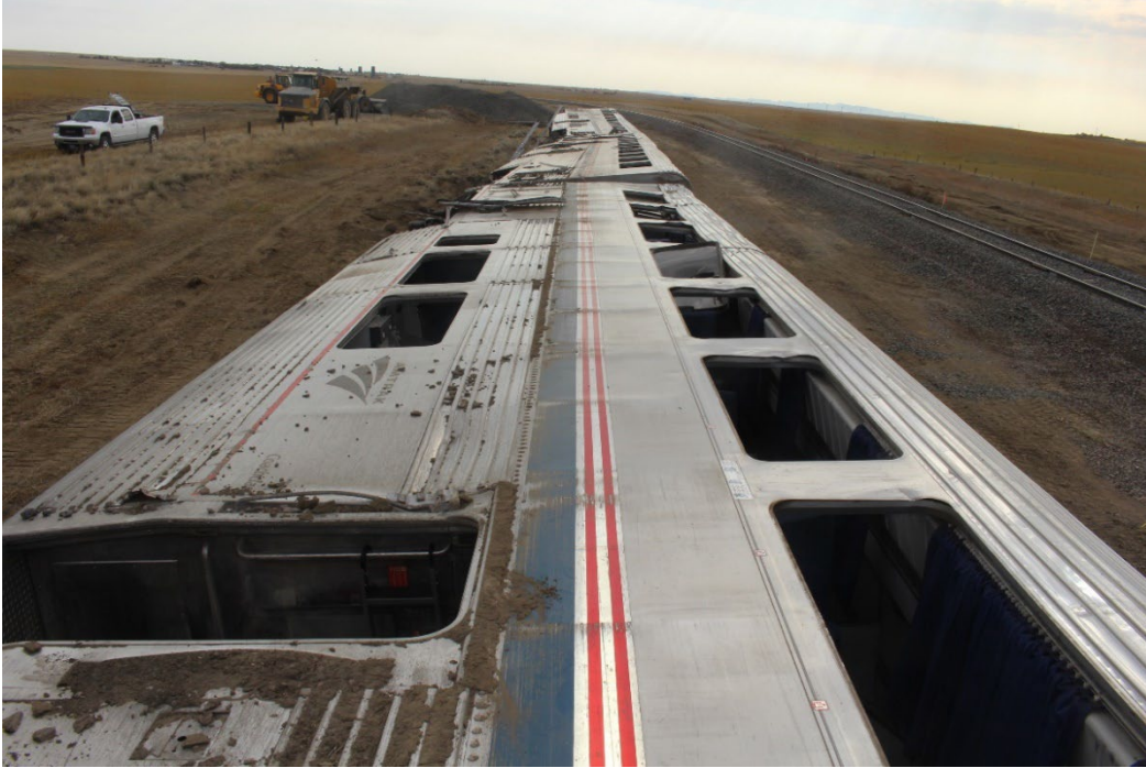
Figure 11 Photograph taken from the top (right) side of the three uncoupled train cars that overturned east of the main train body. The train cars were flipped onto their left side during the search for victims. (Source: NTSB)
