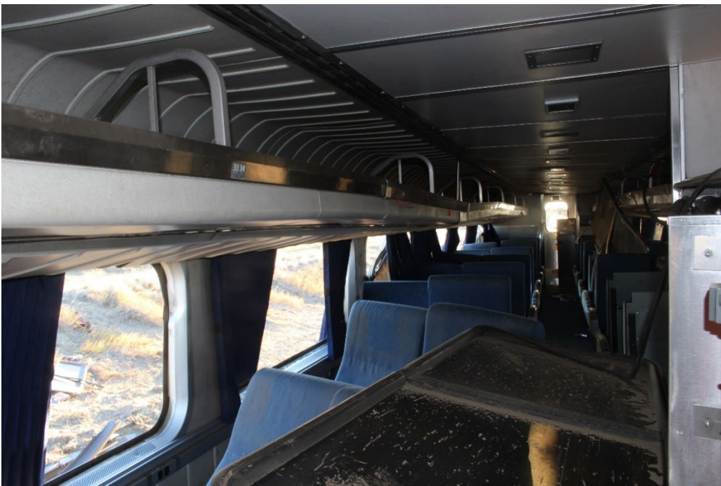
Figure 14 Photograph of the interior of Coach Car ATK 31036 showing the damage sustained in the derailment to include deformation to spaces above train seats caused by impact with passenger heads and missing and removed windows. (Source: NTSB)
