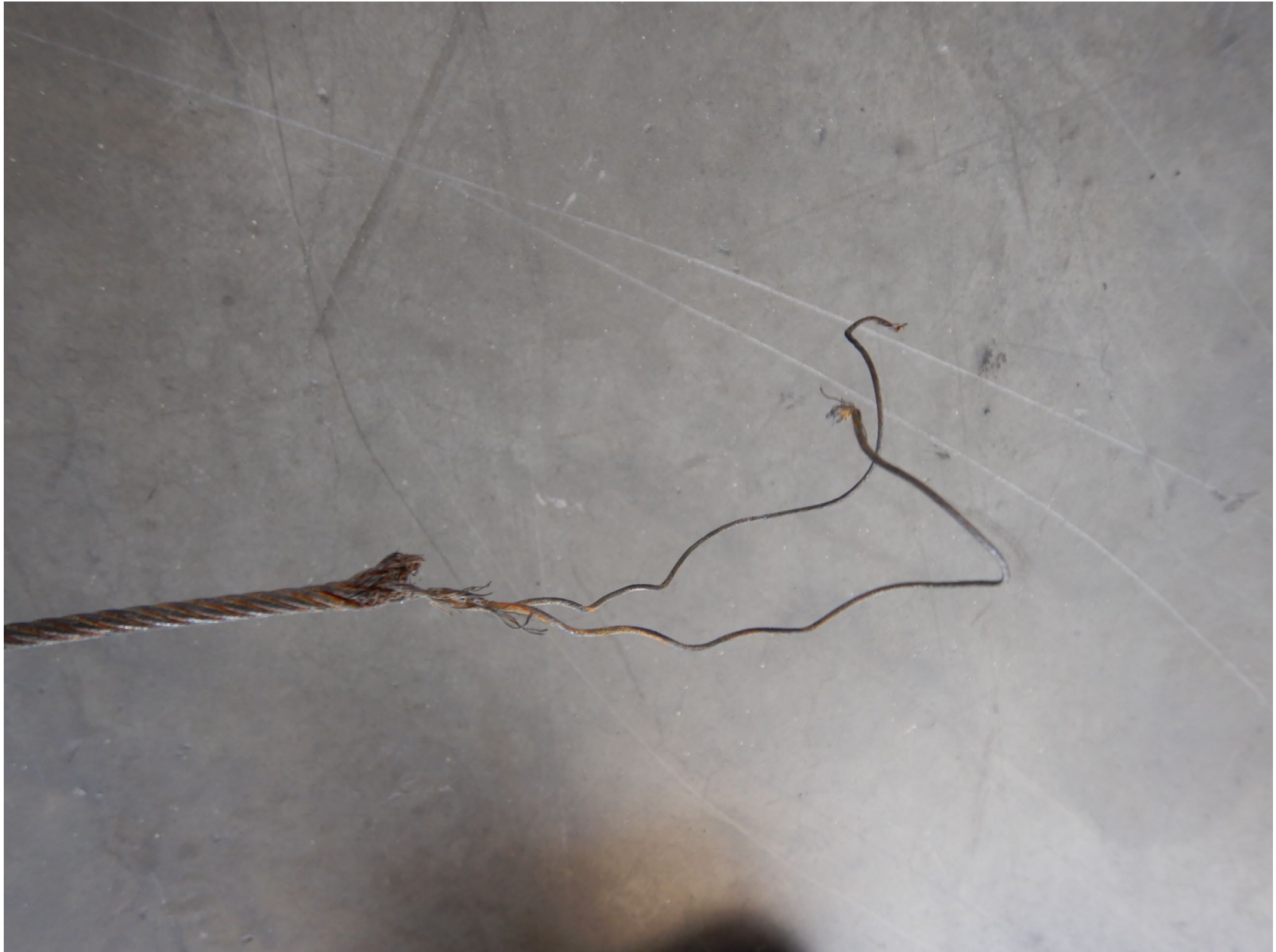
Photo 5 -Aileron carry-through cable
