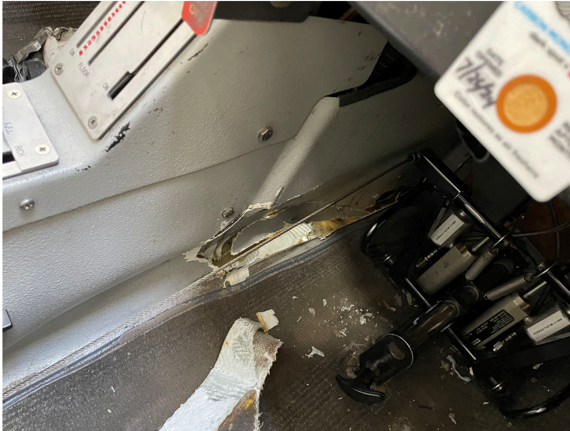
Photograph 2 - Photo showing substantial damage to the floor (Courtesy of the operator)
