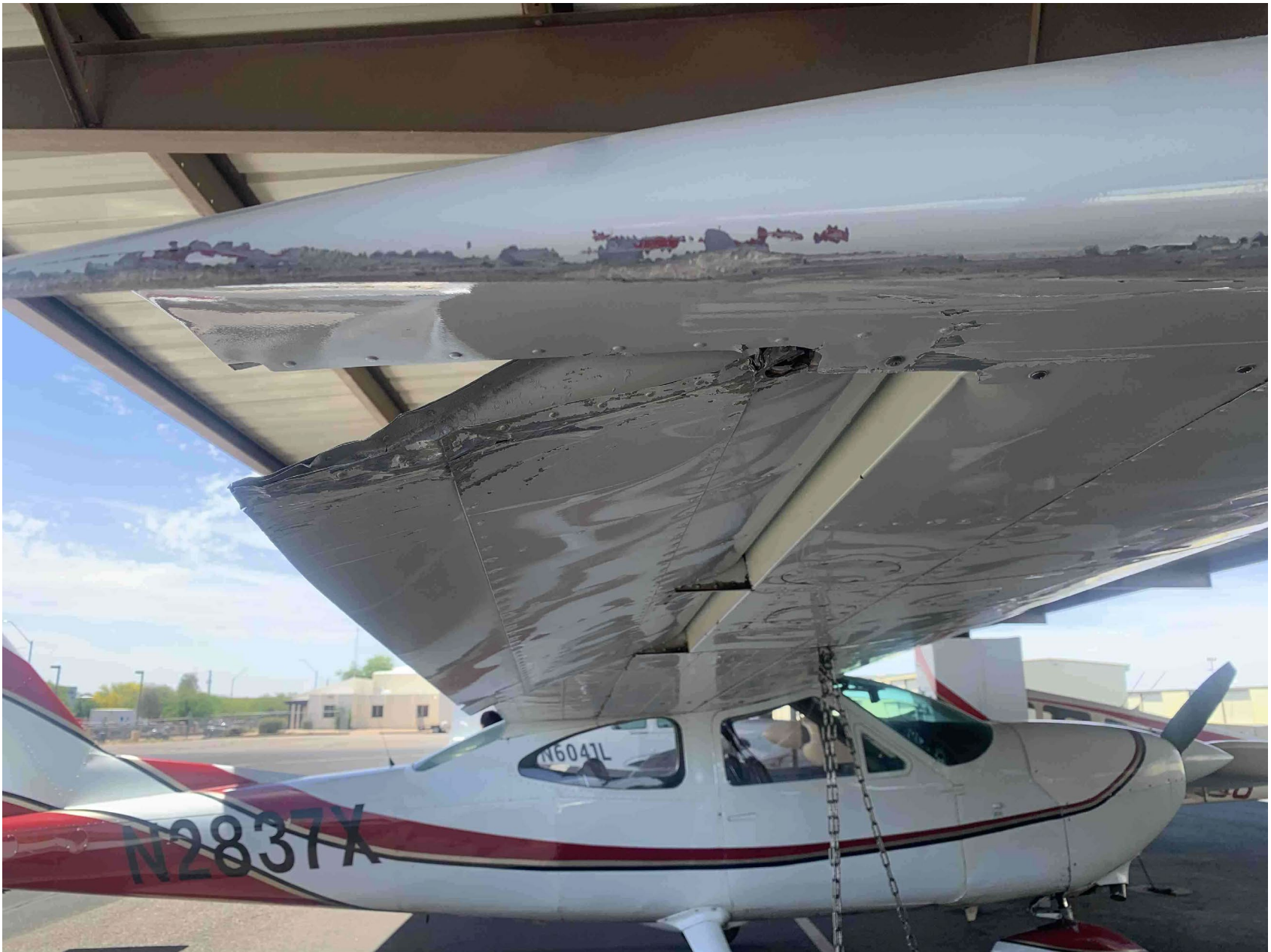
Photo 1 – Right Wing Aileron Damage (Photo courtesy of flight instructor)
