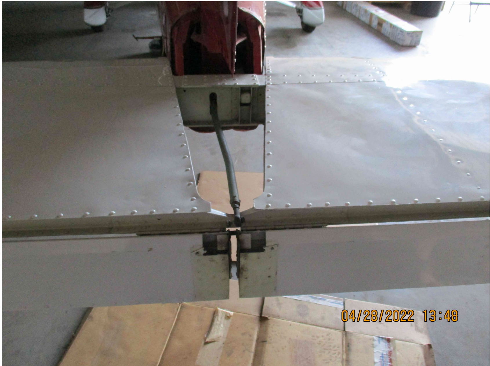
Photo 2 – Stabilator damage from rear (Photo courtesy of aircraft owner)
