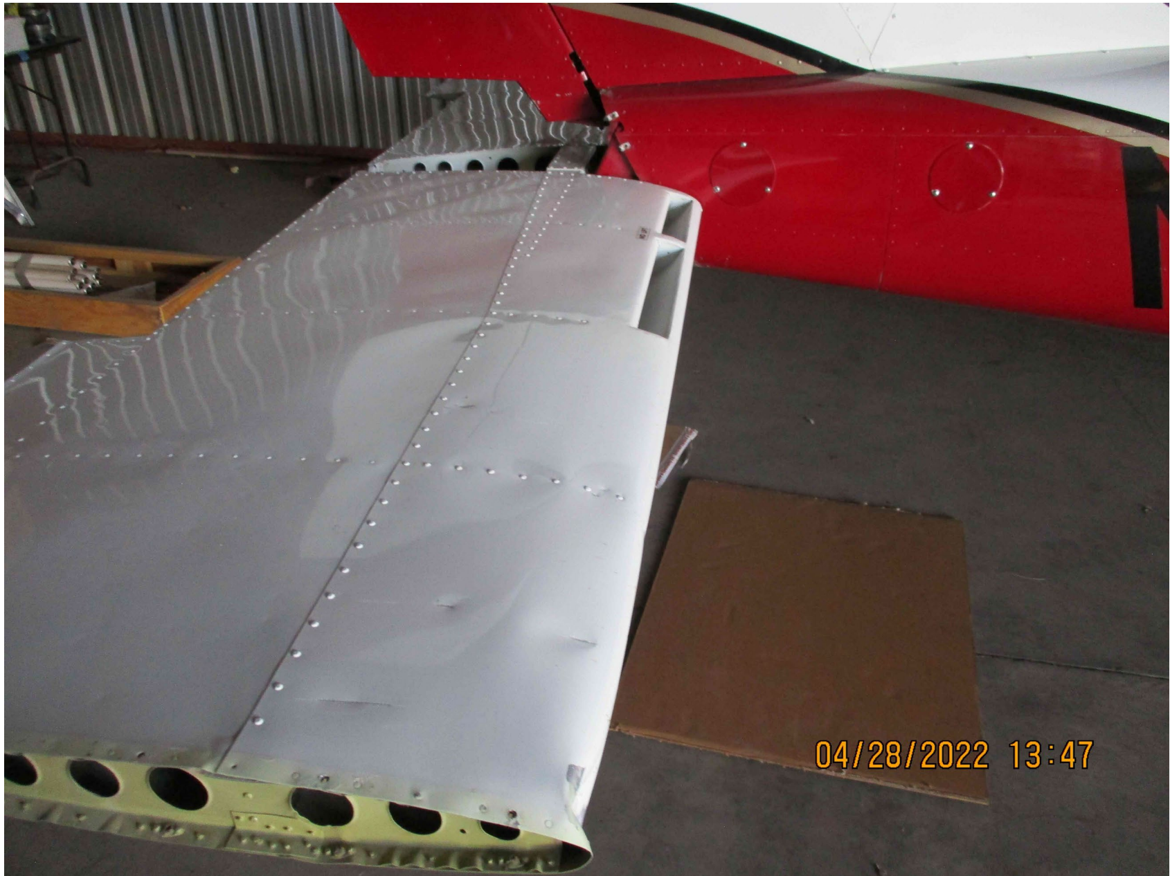
Photo 3 - Stabilator damage right side (Photo courtesy of aircraft owner)
