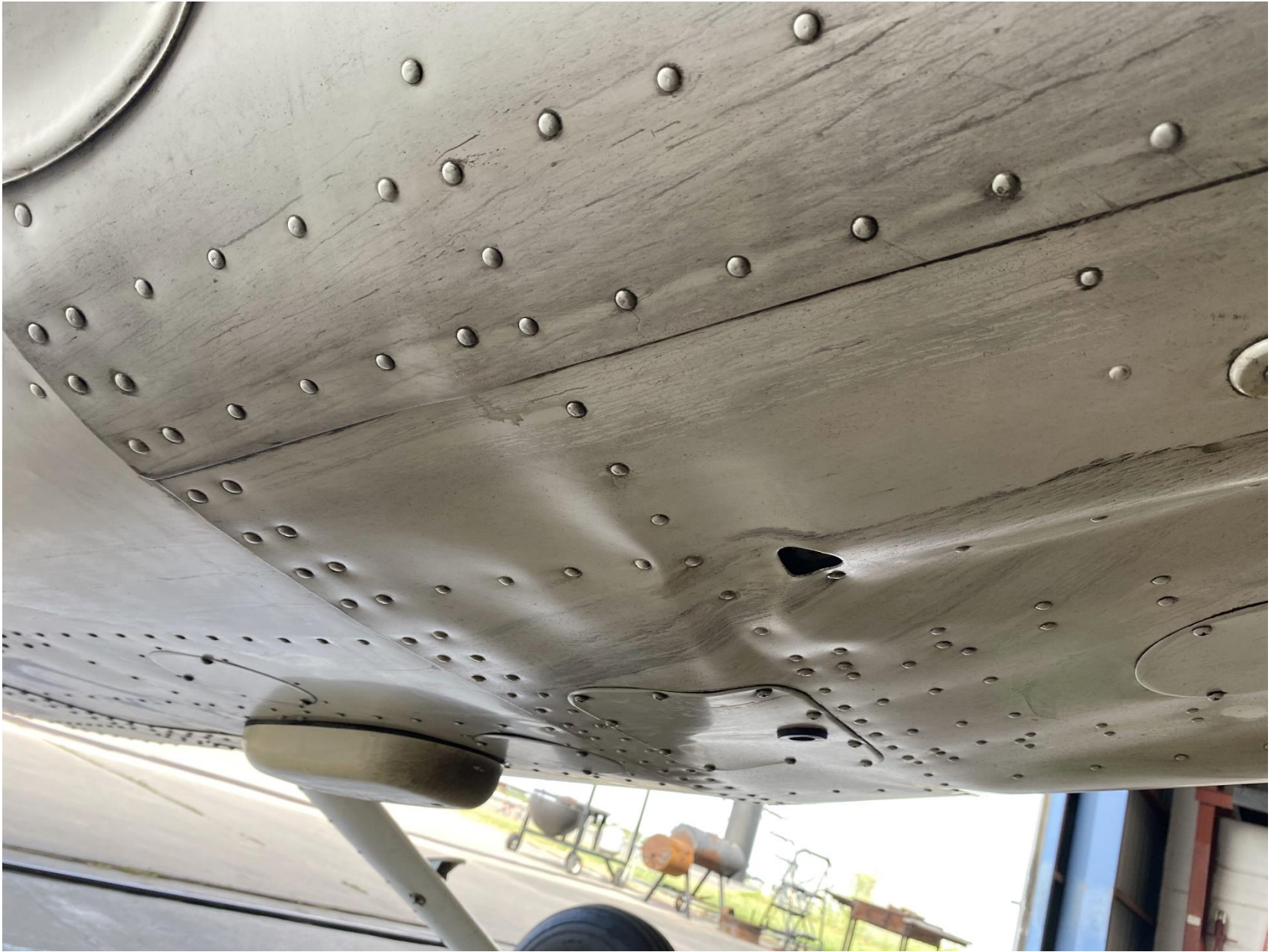
Photo 1 – Lower Fuselage Damage (Flight School photo)
