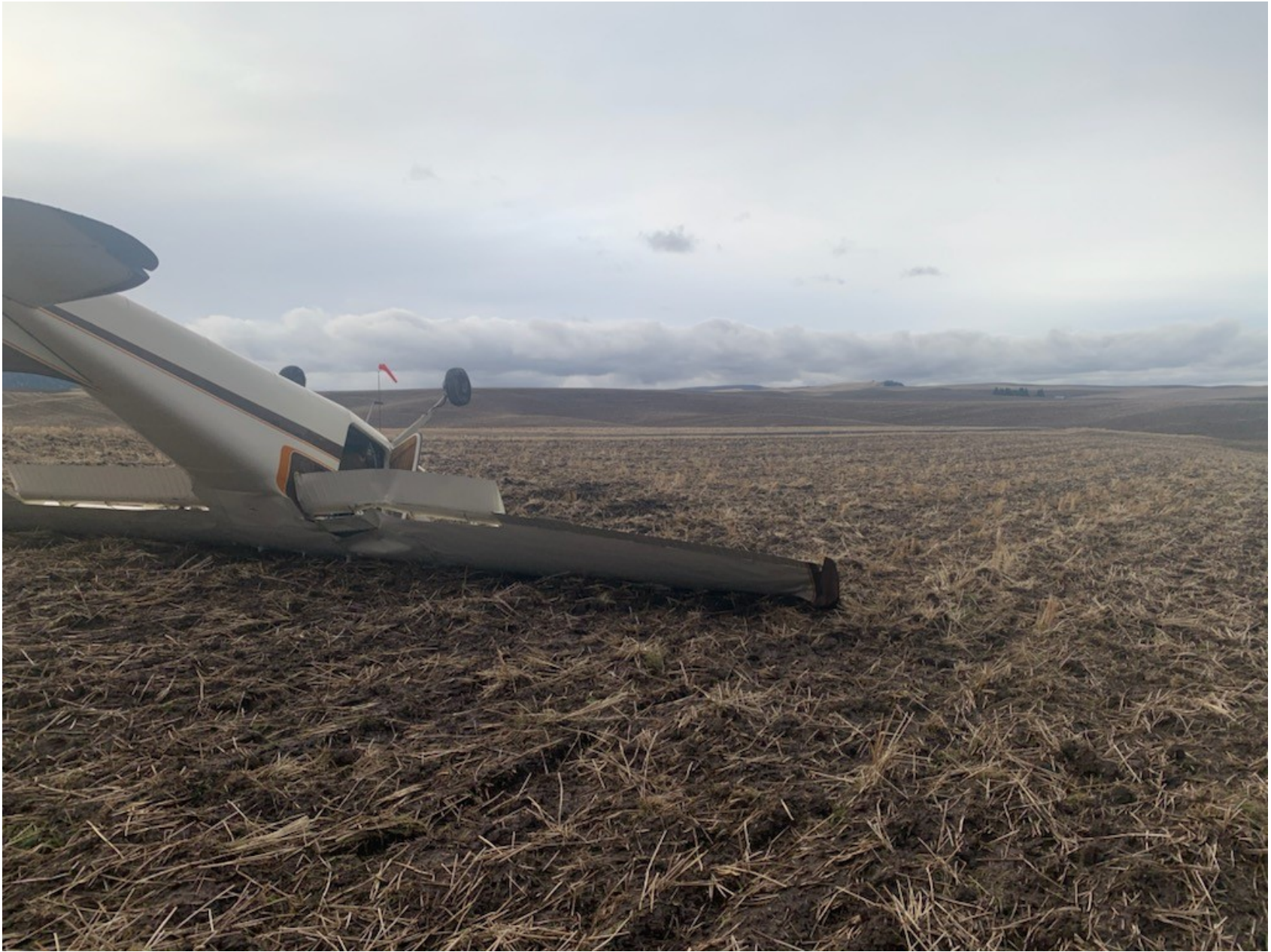
Photo 2 – View of damage to left wing
